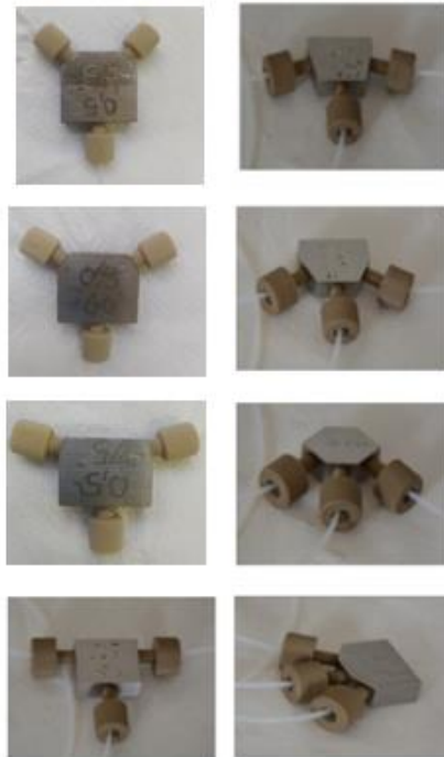
Figure 2.9 : Micromixers angles design.
