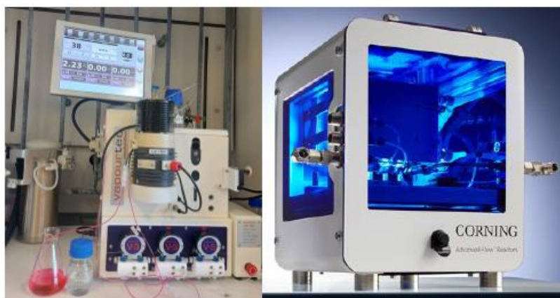
Figure 1.16: Integrated systems in continuous flow: Vapourtec® (left) and Corning® (right)
