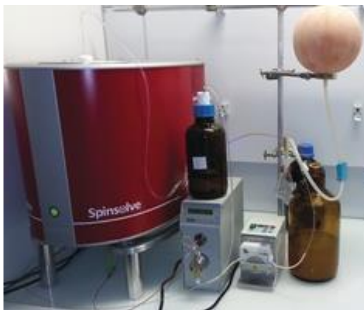
Figure 1.19: Real photo of NMR inline (excerpt from Picard et al. 2017). 32
