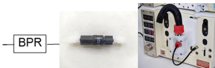
Figure 1.14: BPR symbol (left), image (middle), heated back pressure regulator assembly (right).
