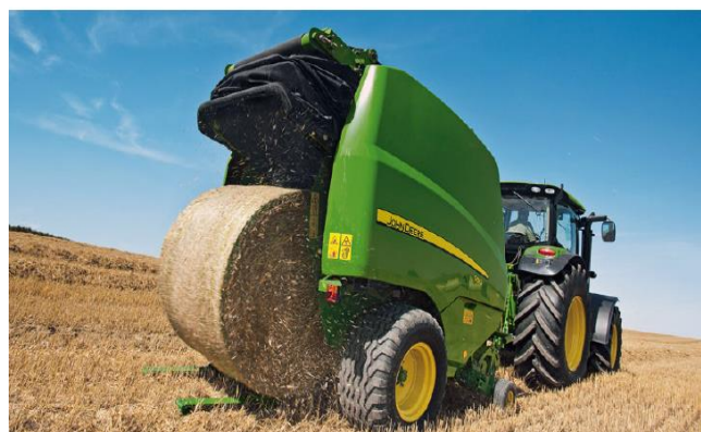
Figure 6.2: High-density round baler from John Deere 900 [119]
