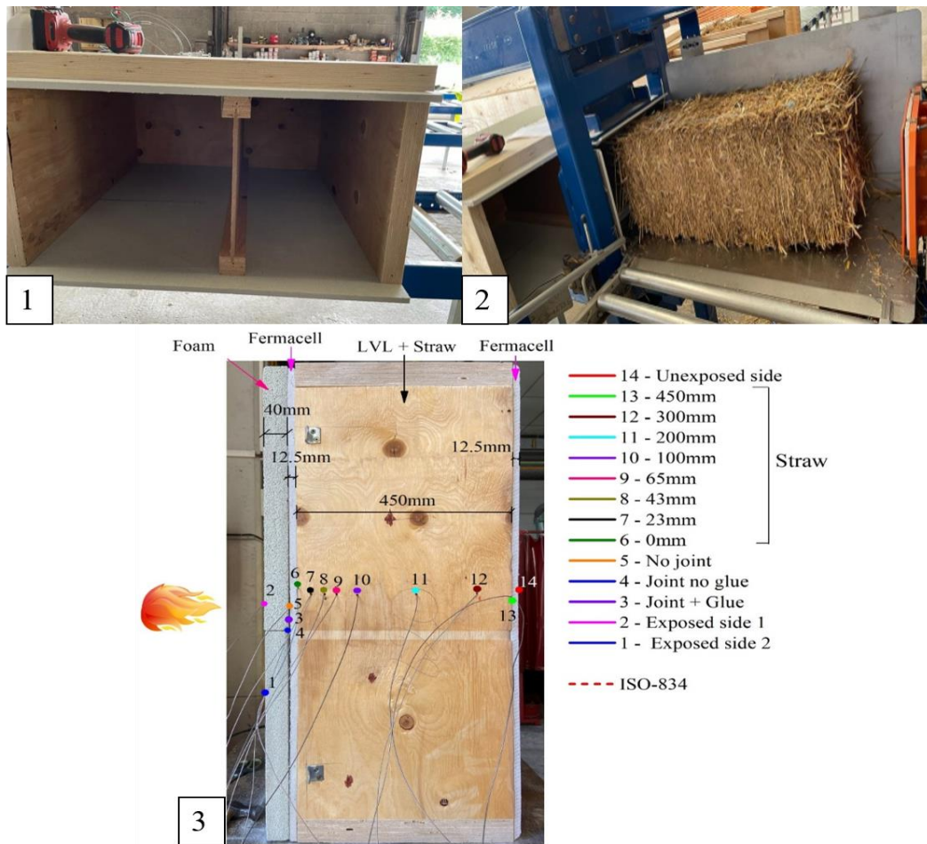
Figure 8.2: Sample preparation steps and the thermocouple placement inside and on the surfaces of the wall
