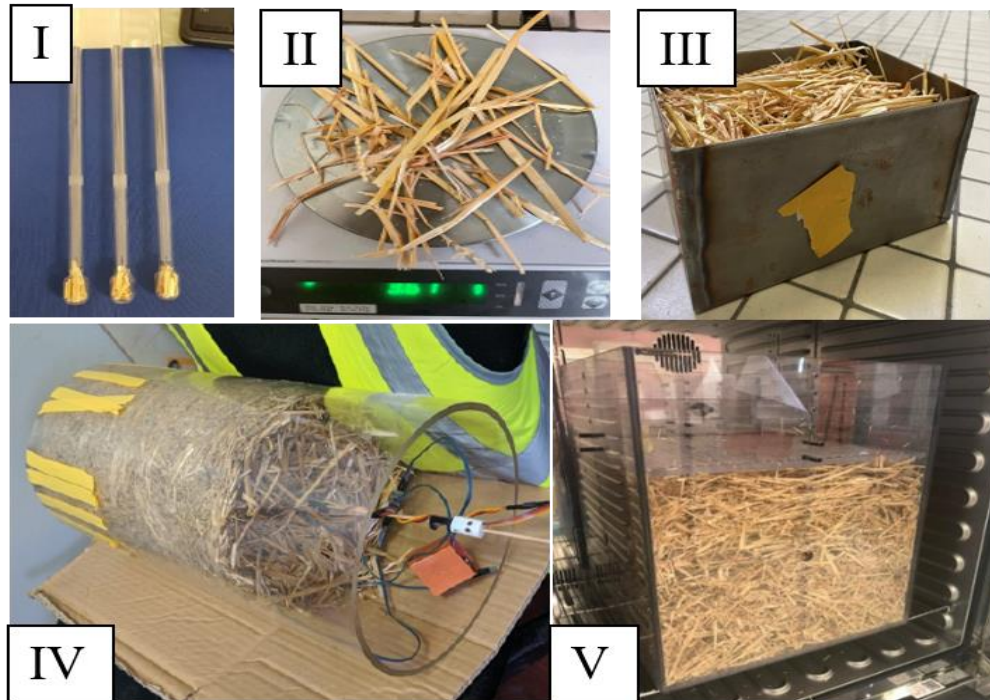
Figure 6.4: Different types of samples used in the experiments. Samples I and II are fibers, and III, IV, and V are bales with different dimensions and densities
