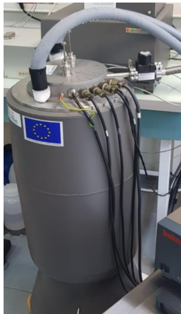
Figure 6.15: Calvet cryo calorimeter
