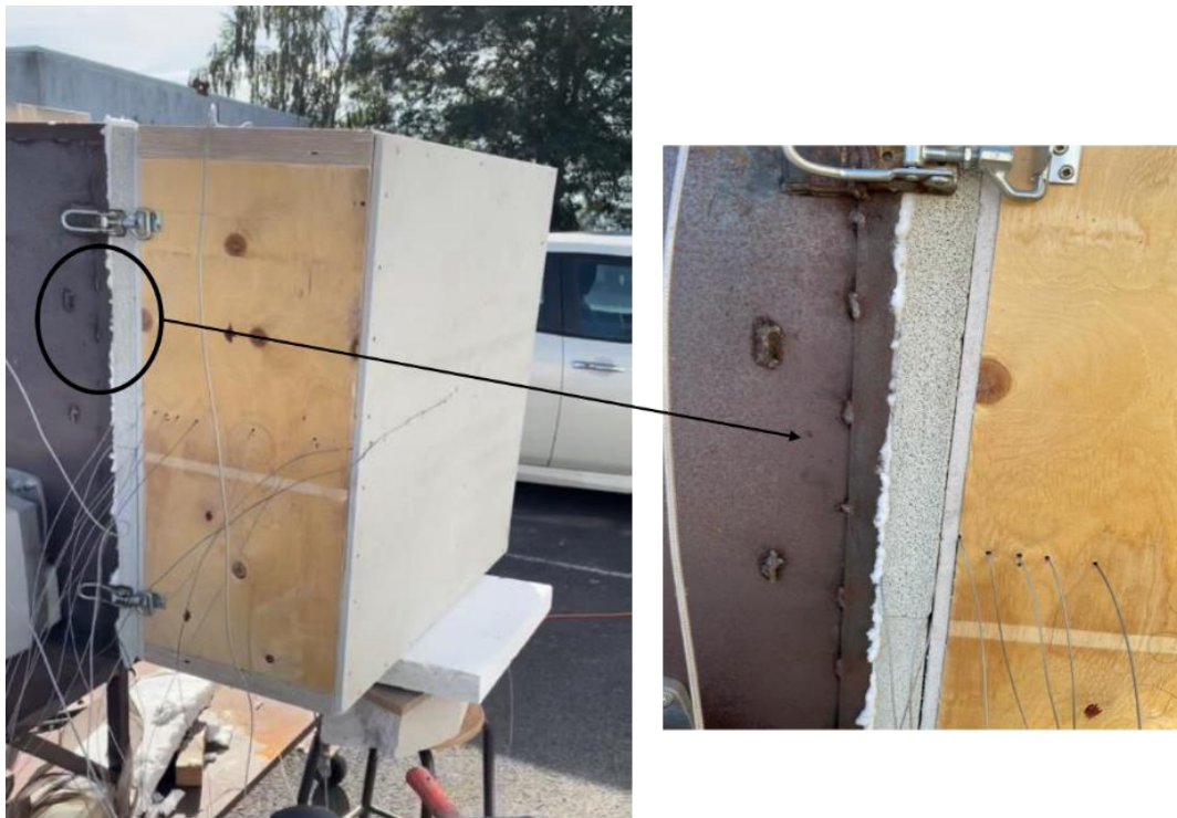
Figure 8.5: Installation of a straw wall. Insulation material is added at the edges between the wall and the furnace before starting the experiment
