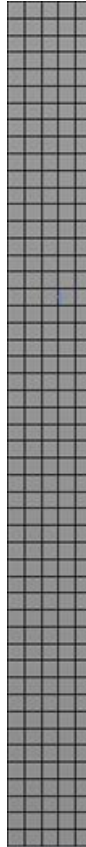
Figure A.1: Rectangular bubble column with a constant mesh size of 2 cm
