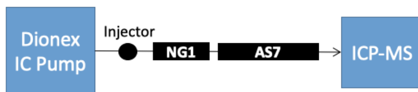
Figure 17. Setup for preliminary studies with the Dionex Ionpac AS7 ion-exchange column.
