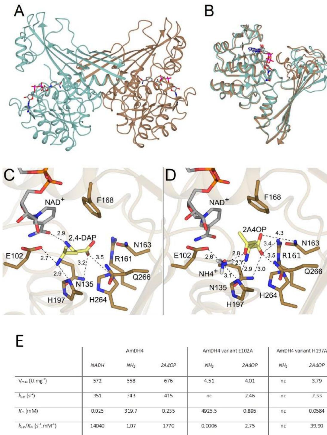
**Figure 2. Structural and mutagenesis data of AmDH4.** **A:** Structure of dimer of AmDH4 consisting of one open and one closed form; **B:** Superimposition of open and closed monomers of AmDH4 in blue and brown respectively; **C:** Active site within closed form of AmDH4 with product 2,4-DAP modeled
