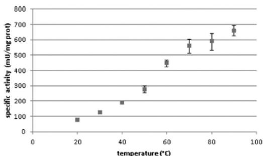
Fig. 2 Profile of activity versus temperature for AmDH4 on 4-oxopentanoic acid (6). Reaction conditions: 300 mM  $\text{NH}_4\text{Cl}/\text{NH}_4\text{OH}$  buffer, pH 7.2, 200  $\mu\text{M}$  NADH, 100 mM 6. Error bars represent the standard deviation of three independent experiments.
