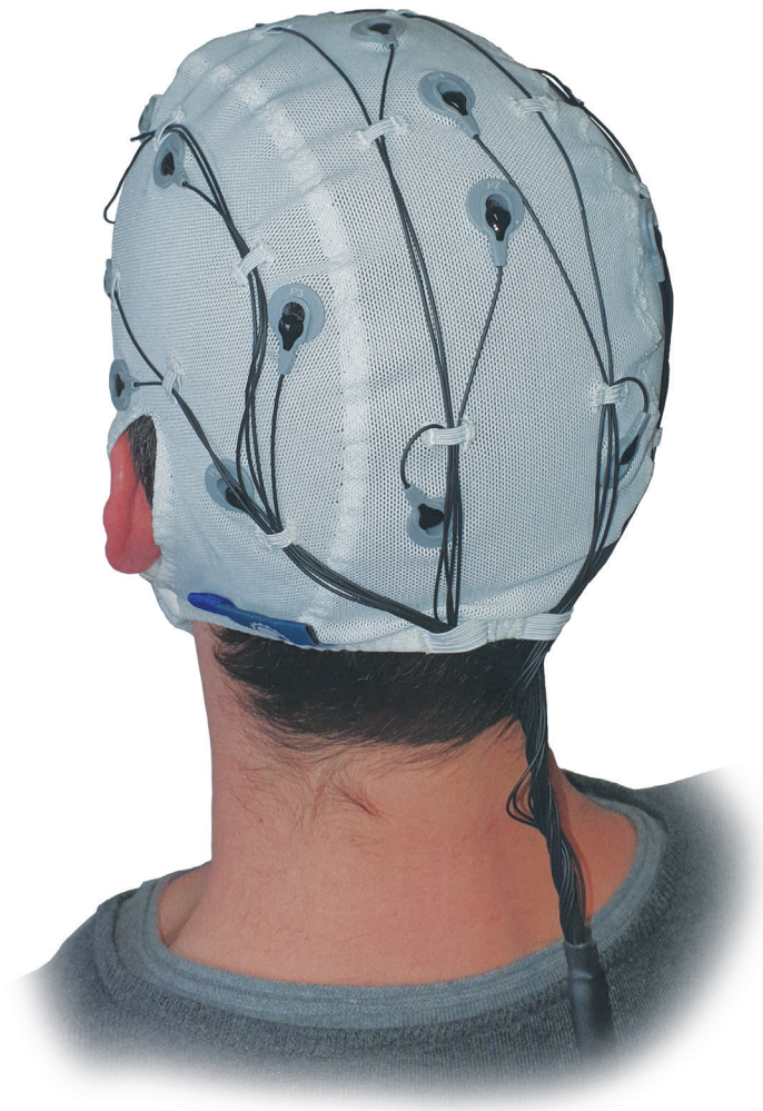
Figure 3.5. 16 electrodes OpenBCI EEG cap.
