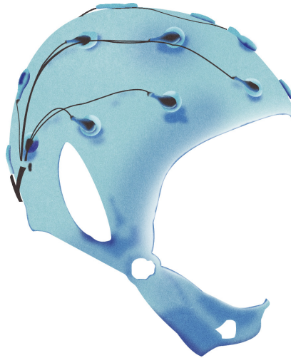
Figure 2.4. Example of an ElectroEncephaloGraphy cap with 16 electrodes.
