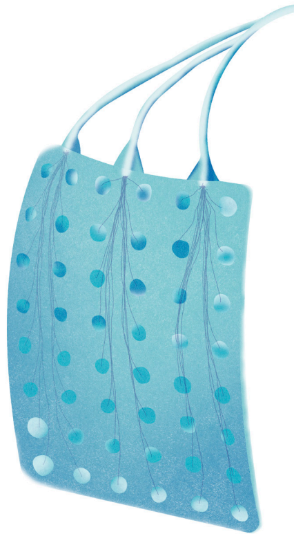
Figure 2.3. Example of a flexible ElectroCorticography array of electrodes. The array can be placed either under or over the dura mater.
