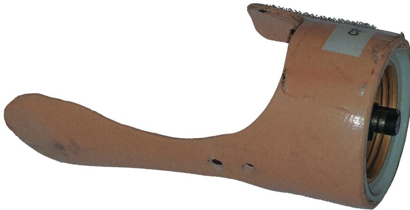
Figure 4.4. Myobock socket used at the IRMA to quickly test the prosthesis on the patients.
