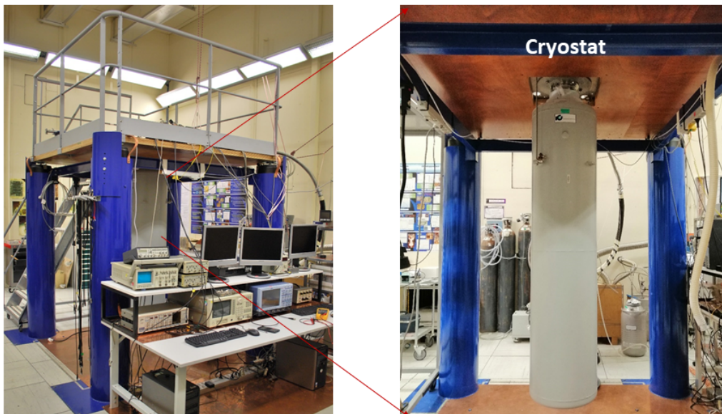
Figure 3.30: Installation of cryostat at LNHB.
