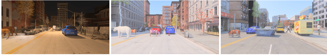
Figure 2.5: Illustration of images with OOD examples from MUAD dataset. The three images are selected from the OOD set . The animal, rocks, trash bags, and food track are the OOD examples.
