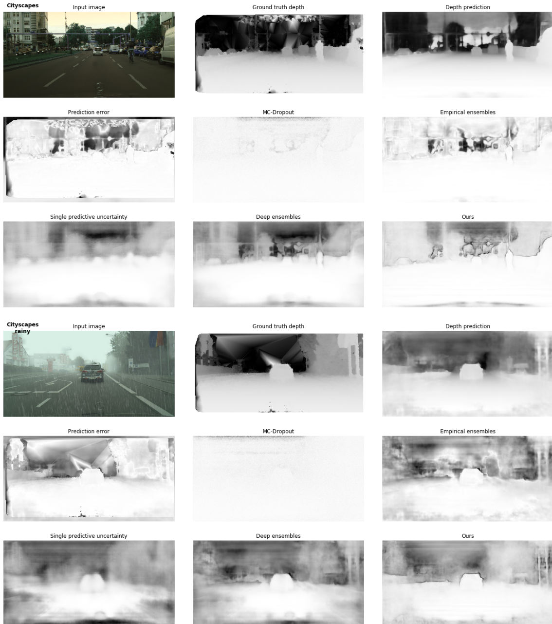
Figure 3.7: Uncertainty estimation results for monocular depth estimation task. The ground truth maps are rebuilt by interpolation just for visualization. For uncertainty maps, black indicates higher uncertainty, and white indicates lower uncertainty. For depth maps, black represents deeper depth, and white represents shallower depth.
