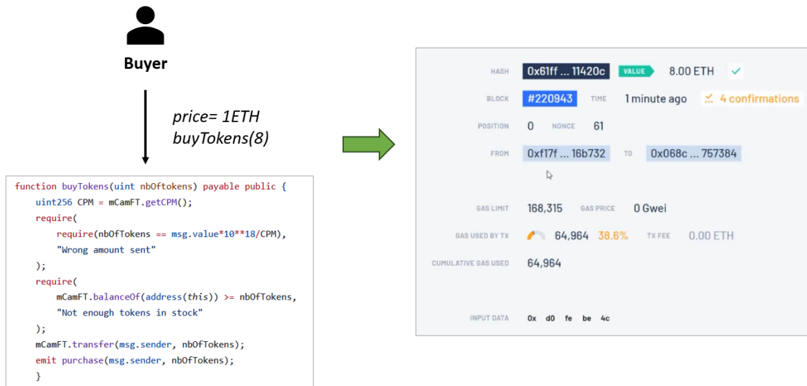
Figure 50: Illustration of a transaction to the buyTokens() function (bottom left) and resulting transaction observed on our private blockchain (right).
