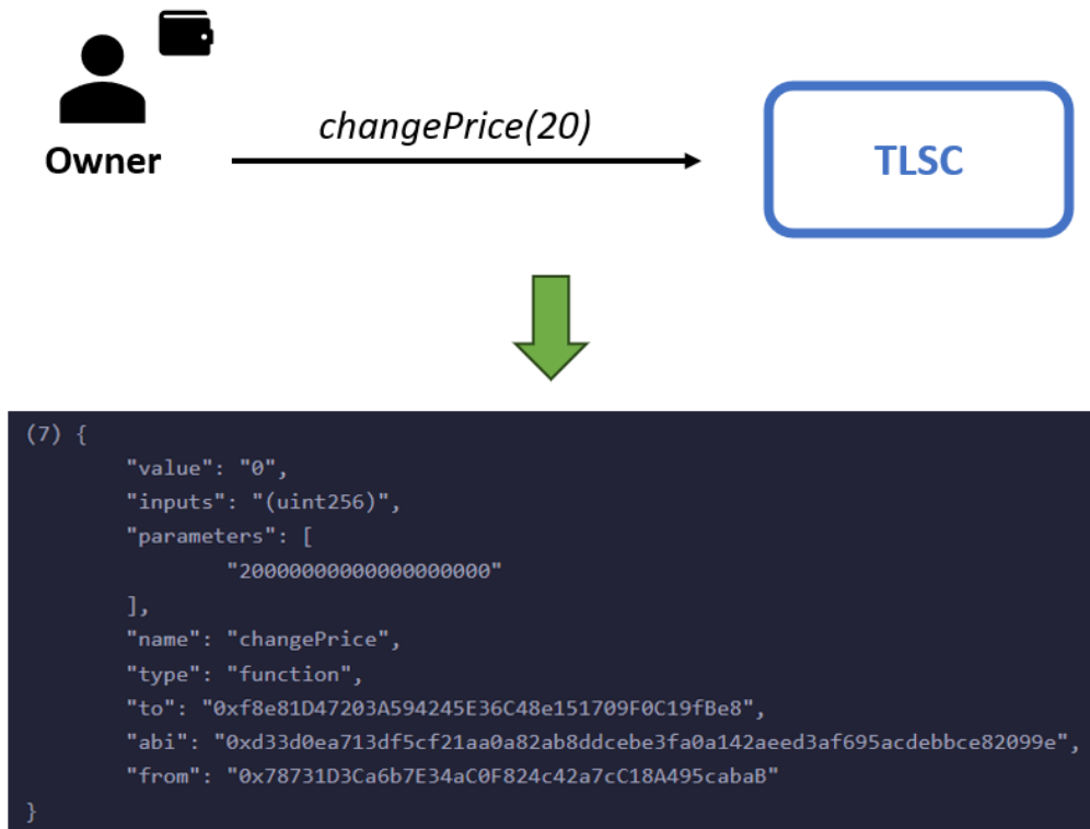
Figure 55: The receipt of an Ethereum transaction to the changePrice() function of a Token Level Smart Contract (TLSC).
