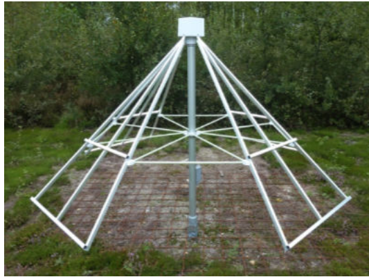
Figure 2.3: Photo of an antenna of NenuFAR. (© Observatoire Radioastronomique de Nançay)
