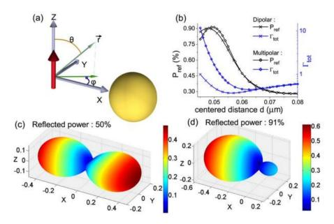
Figure 1-10. Emitter modelled as point dipole with tangential orientation and 80 nm AgNP –(a). Reflected power (black) and total decay (blue) as distance from AgNP varies using dipolar approximation (cross) and multipole expansion (diamonds)- (b). 3D plots of radiation pattern at 19 nm (c) and 9 nm (d) from the surface [ $^{130}$ ].
