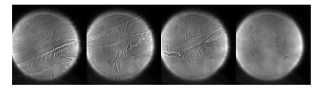
Figure 2-21. The evolution of pT matrix morphology (left to right) when moving along (2x) and perpendicularly (1x) to the long axis of the very thin islands.
