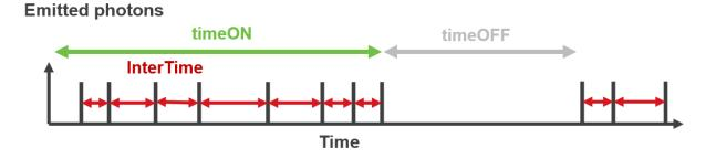
Figure 1-15. Exemplary behavior of photon emission events in time and telegraph parameters such as InterTime – time between subsequent photon emissions, timeON – interval of repeatable photon emissions and timeOFF – interval of no photon emission events.
