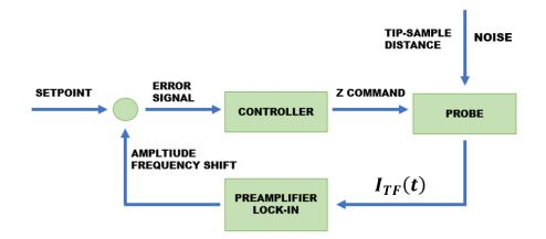
Figure 2-13. Closed-loop feedback in SPM control system using Tuning Fork probe.
