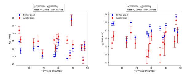
Figure 3-21. Spontaneous emission rate  $(k_{21}, left)$  and singlet excitation coefficient  $(\sigma_{12}, right)$  for 16 spectrally selected molecules calculated using Power Scan (blue dots) and Polarization Scan (red dots) cos<sup>2</sup> approximation. Error bars given by fit uncertainty.
