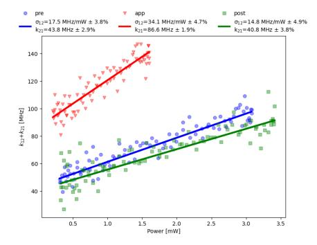
Figure 4-7. Sum of the excitation rate  $(k_{12})$  and spontaneous emission rate  $(k_{21})$  as a function of the excitation laser power. The pre-approached (blue dots), approached (red triangles) and post-approached (green squares) with linear fits (lines) and fit parameters given in the inset.
