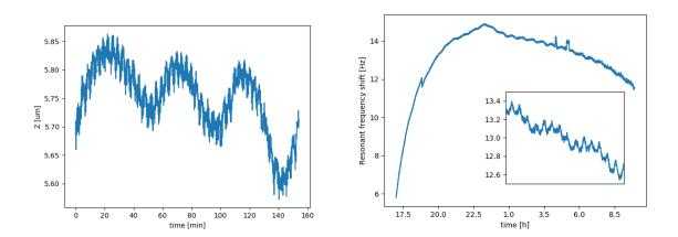
Figure F-1. Height profile of tip scanning on repeat sub-40 nm pT matrix – high-frequency component due to the matrix height variations, slow frequency due to the drift of TSD (left). Probe's fres overnight in the retracted state; inset shows the zoomed range at night (right).
