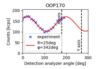
Figure 3-22. Analyzer Scan of E170 species with fitted polar and azimuthal angles ( $\theta = 25 \text{ deg}$ ,  $\varphi = 342 \text{ or } 162 \text{ deg}$ ); datapoints (blue crosses) and fit (red line). Axis of the cartesian coordinate system are given with dashed lines.
