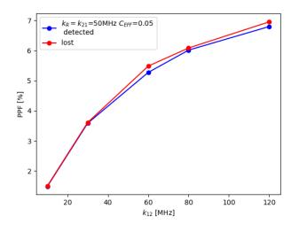
Figure 2-6. PhotonPair Fraction (PPF) for a near-unity quantum yield emitter at  $C_{EFF}$ =0.05 and  $k_{21}$ =50 MHz as the function of  $k_{12}$  that was detected (blue) and lost in the deadtime (red).
