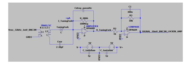
Figure 2-15. LT Spice scheme of the designed preamplifier.
