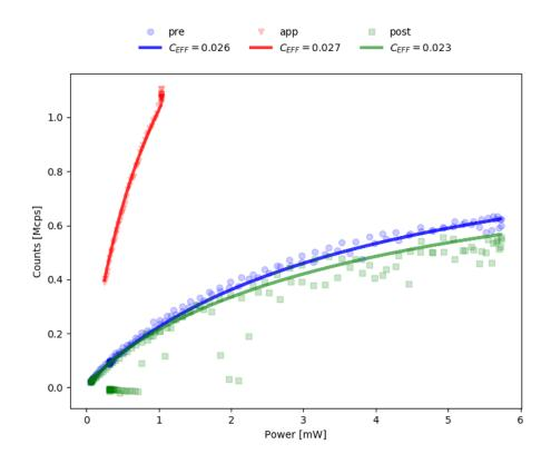
Figure 4-22. Background corrected counts on the detectors as a function of the excitation laser power. The pre-approached (blue dots), approached (red triangles) and postapproached (green squares) with counts calculated from the rates and corrected for the deadtime (lines) and adjusted collection efficiency given in the inset.
