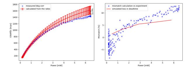
Figure 3-9. Counts calculated from the rates and experimental (left) and mismatch between the two (right) overlaid with the loss predicted by the simulation due to the detector deadtime.
