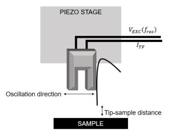
Figure 2-12. Shear force AFM configuration (center).
