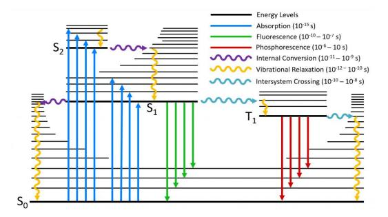
Figure 1-1. Jablonski diagram showing common photophysical processes in a single molecule and their typical time in the legend. Processes involving photons are illustrated using straight lines, while non-radiative process are depicted using wavy lines. [<sup>8</sup>].
