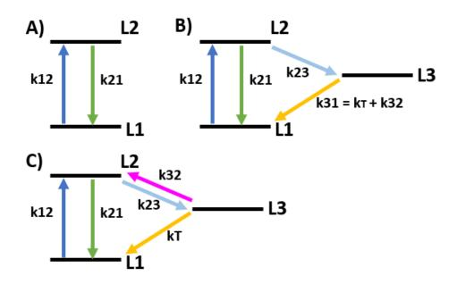
Figure 1-14. Typical mathematical models used in photon statistics studies: 2-level system (A), 3 level with uni- (B) and bidirectional (C) pathway between levels 2 and 3.
