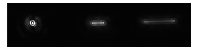
Figure 2-18. Images on the camera (tip with red diode coupled into fiber) at excitation of 0 V, 1 V and 3 V (left to right) applied to the probe of Q=2000 and fres=32,6 kHz.
