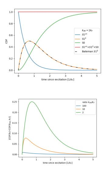
Figure A-1. Transient probability of states occupancy as a function of time since molecule was excited to the vibrational level of the excited singlet  $S1^{\nu_N}$  (upper) and transient absolute error when a sequential process is approximated with the slower process only for different ratios of the rates.
