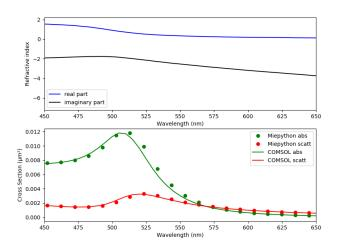
Figure 1-7. Real and imaginary part of refractive index (upper) [<sup>112</sup>] used for the calculations of 80 nm gold nanoparticle absorption and scattering cross-sections using analytical solutions from Mie theory (Miepython package) and COMSOL software.
