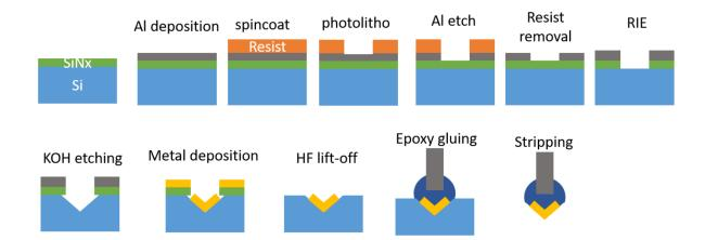
Figure I-1. Scheme of the fabrication protocol [185].
