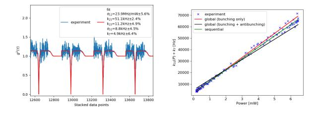
Figure G-2. Zoomed-in region of the stacked antibunching and bunching global fit (upper). The comparison of the global using bunching part only (red line) or antibunching and bunching part (black line) and sequential fit (green line) with the experimental data (blue crosses).
