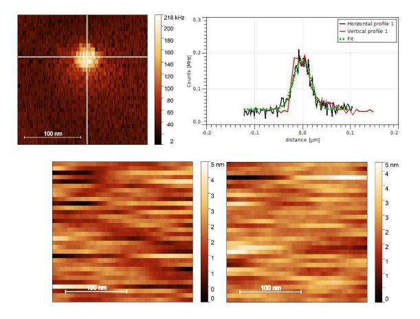
Figure 4-2. Counts on the detector as the dielectric tip is scanned above a single T in sub-30 nm pT (upper left). The PSF's vertical and horizontal cross-sections with a Gaussian fit that yields 45 nm FWHM (upper right) and counts enhancement of ~3. Back and forth height images of the same area (lower) recorded simultaneously.
