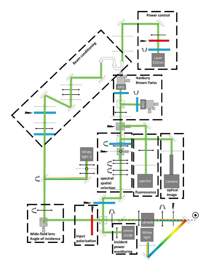
*Figure 2-2. Scheme of the optical set-up with particular functionalities marked in dashed boxes with the descriptions.*
