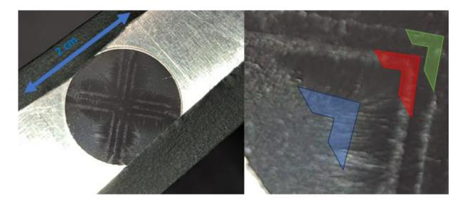
Figure 2-20. Macroscopic morphology of the spin-coated T/pT (left) and zoomed pattern transition of the 2 mg/ml sample (right). Microscope cover plate 2 cm x 2 cm.
