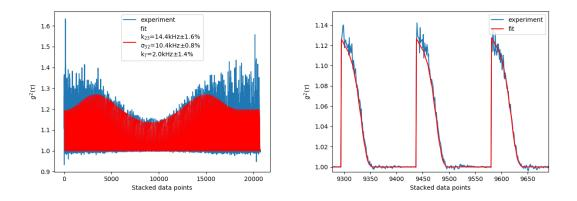
Figure G-1. Global fit of the bunching part – one array made of 145 cross-correlation at different incident power (left) and zoomed-in region (right).
