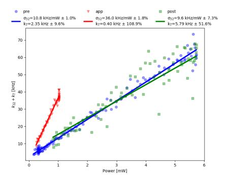
Figure 4-20. TimeOFF as a function of the excitation laser power. The pre-approached (blue dots), approached (red triangles) and post-approached (green squares) with linear fits (lines) and fit parameters given in the inset.
