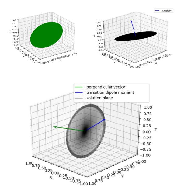
Figure 3-16. Exemplary representation of the polarization plane as  $\alpha_{EXC}$  rotates by 360 deg (upper left). An arbitrary transition moment with its perpendicular plane (upper right). An arbitrary transition moment with its perpendicular vector, which is a normal vector to the solution plane that contains this transition dipole moment (bottom).
