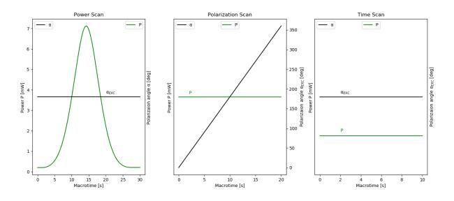
Figure 2-8. Incident excitation power (P) measured on the photodiode and the excitation laser polarization angle ( $\alpha_{EXC}$ ) during Power Scan (left), Polarization Scan (center) and Time Scan (right).
