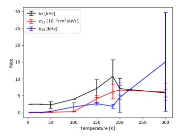
Figure 1-6. Average rates describing T1 population ( $k_{23}$ ), depopulation to S0 ( $k_T$ ) and crosssection of the transition providing depopulation to S1 ( $\sigma_{32}$ ) in T/pT measured at different temperatures [<sup>45</sup>]. Error bars calculated from their population standard deviation. Original units from the reference kept, regardless of unit conversion error suspected.
