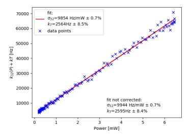
Figure 3-4. Sum of the  $k_T + k_{32}$  as a function of the power assigned to each time segment, data points (blue crosses) and the fit (red line). Results of the linear fit  $\sigma_{32} * P + k_T$  in the caption and without background correction in the text (right).
