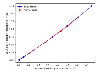
Figure 2-7. Counts corrected for deadtime as a function of counts measured by a detector with 90 ns deadtime according to the Monte Carlo simulation and Sontheimer [<sup>160</sup>].
