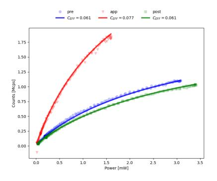
Figure 4-10. Counts on the detectors as a function of the excitation laser power. The preapproached (blue dots), approached (red triangles) and post-approached (green squares) with counts calculated from the rates and corrected for the deadtime (lines) and adjusted collection efficiency given in the inset.
