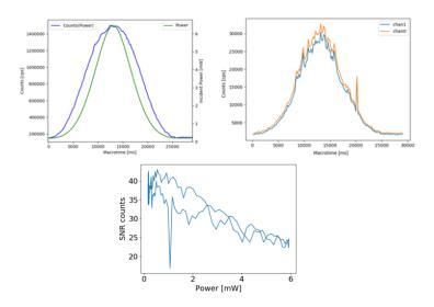
Figure 3-1. Counts on each channel (detector) from the single T/pT (upper left), pT taken a few  $\mu$ m away from the emitter (upper right) and SNR being the ratio of both (lower) as a function of power during Power Scan.
