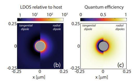
Figure 1-9. Relative LDOS (left) and modified QY (right) of a perfect unity QY emitter around 100 nm AuNPs for tangential and radial dipole orientation (emission wavelength 600 nm) [<sup>141</sup>].
