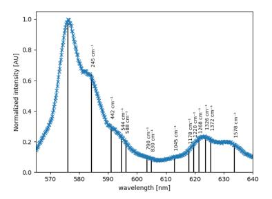
Figure 1-4.Experimental fluorescence spectrum of T/pT with vibrations assigned according to the reference [<sup>28</sup>] and taking 576 nm as 0-0 transition line. Vibrations closer than 20 cm<sup>-1</sup> to each other were reduced to single vibration for clarity.
