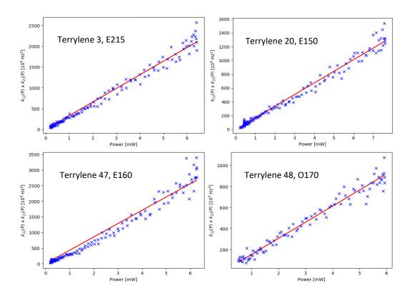
Figure 3-30. Product of excitation rate and intersystem crossing rate (k12 \* k23) for 4 molecules treated with joined fit. Linear fit (red line) and data points (blue crosses).
