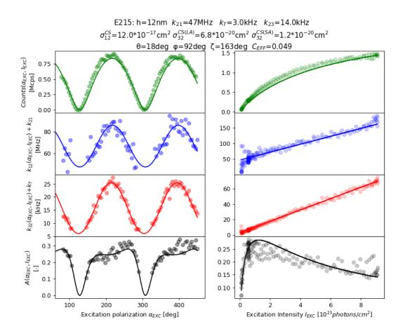
Figure 3-28. Joined fit  $(\sigma_{12}^{CS}\text{-fixed})$  – Angle (left) and Power Scan (right) fit of species E215. In top-down order: counts( $\alpha_{EXC}$ ,  $I_{EXC}$ ),  $k_{12}(\alpha_{EXC}$ ,  $I_{EXC}$ ) +  $k_{21}$ ,  $k_{32}(\alpha_{EXC}$ ,  $I_{EXC}$ ) +  $k_T$  and ( $\alpha_{EXC}$ ,  $I_{EXC}$ ). Parameters of the fit are shown in the header of the figure. Data points in circles and model response in lines.
