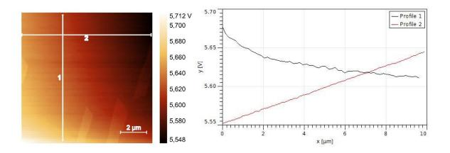
Figure 2-22. Z-command voltage image (left) with cross-section lines and voltage profiles of those lines (right).
