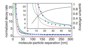
Figure 1-12.Radiative, non-radiative and total decay rates (green, pink and blue) calculated for T tilted at 15° and experimental data points (blue circles) as a function of the distance between the molecule and 100 nm AuNP nanoantenna. Inset shows zoomed range up to 50 nm and calculated QY (black line) [<sup>114</sup>].
