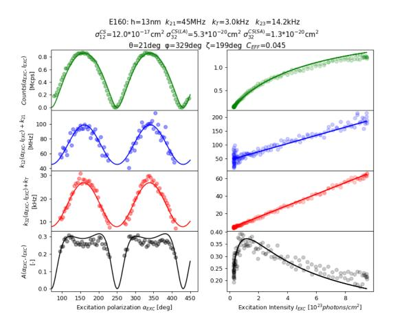
Figure 3-29. Joined fit ( $\sigma_{12}^{CS}$ -fixed) – Angle (left) and Power Scan (right) fit of species E160. In top-down order: counts( $\alpha$ \_EXC,I\_EXC), k\_12 ( $\alpha$ \_EXC,I\_EXC)+k\_21, k\_32 ( $\alpha$ \_EXC,I\_EXC)+k\_T and ( $\alpha$ \_EXC,I\_EXC). Parameters of the fit are shown in the header of the figure.
