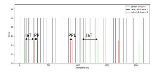
Figure 2-4. Timetrace (bin size 1 ns) of simulated photon flux showing photons emitter by an emitter (grey), photons detected on channels 0 and 1 (green and red), Interchannel time
