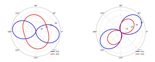
Figure 3-20. Polar plots of the singlet and triplet excitation rates ( $k_{12}$  and  $k_{32}$ ) showing the odd group (left) and the even group (right).
