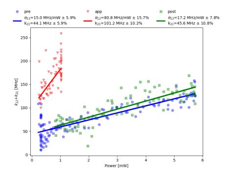
Figure 4-19. Sum of the excitation rate  $(k_{12})$  and spontaneous emission rate  $(k_{21})$  as a function of the excitation laser power. The pre-approached (blue dots), approached (red 187
