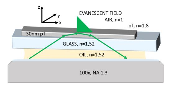
Figure 2-9. TIRF illumination mode and sample configuration.
