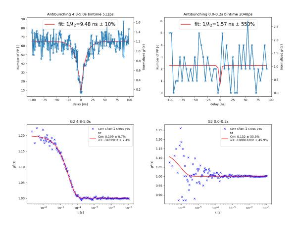
Figure 3-17. Examples of the START-STOP (top row) and cross-correlation (bottom row) at the 1,05 Mcps (left column) and near zero-excitation polarization vector (right column) during Polarization Scan.
