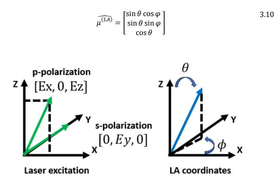
Figure 3-15. Frame of reference – cartesian coordinate system of the experiment with respect to the excitation (left) and the long axis of terrylene expressed in spherical coordinates (right).
