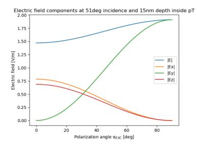
Figure 2-10. Evolution of the electric field amplitude cartesian components as the function of excitation polarization angle  $\alpha_{EXC}$  at 15 nm depth inside pT.
