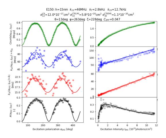
Figure 3-26. Joined fit  $(\sigma_{12}^{CS}\text{-fixed})$  – Angle (left) and Power Scan (right) fit of species E150. In top-down order: counts( $\alpha_{EXC}$ ,  $I_{EXC}$ ),  $k_{12}(\alpha_{EXC}$ ,  $I_{EXC}$ ) +  $k_{21}$ ,  $k_{32}(\alpha_{EXC}$ ,  $I_{EXC}$ ) +  $k_T$  and  $A(\alpha_{EXC}, I_{EXC})$ . Parameters of the fit are shown in the header of the figure. Data points in circles and model response in lines.
