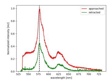
Figure 4-17. Fluorescence spectrum of T/pT with the approached (red) and retracted (green) gold pyramid.
