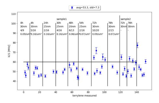
Figure H-1. S1-S0 relaxation rate  $k_{21}$  of T/pT measured with different post-spin coating times and areas of various thickness. X axis represents all of the measured emitters, while fraction given in each columns indicated how many emitters were photostable. Density of number of emitters per area is given with a unit of  $\mu$ m<sup>-2</sup>. Photostable emitters are treated and plotted with error bars being the uncertainty of the fit.
