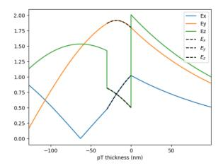
Figure E-1. Comparison of the electric field distribution between analytical solutions and simulation (dashed). The pT film is located bewteen -30nm and 0nm.
