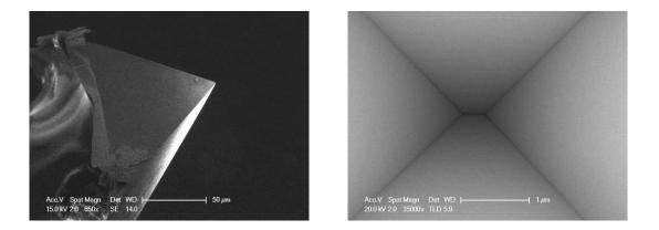
Figure 4-13. SEM images of the pyramids picked-up with the optical fiber and UV glue (left), zoom on the tip of the gold pyramid (base 200  $\mu$ m x 200  $\mu$ m) showing ~200 nm rectangle-like, instead of the point-like apex (right).
