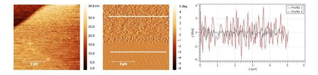
Figure F-4. Height image, phase image and cross-sections of the phase image taken before (Profile 1, black) and after (Profile 2, red) controlled crush, yielding RMS of 0,42° and 1,52°, respectively.
