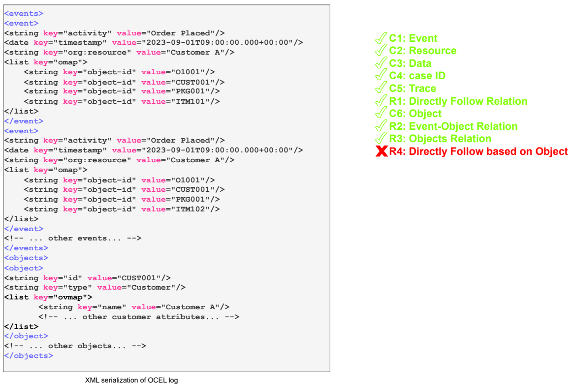
Figure 3.2: OCEL representation of the event log example associated with the order management process
