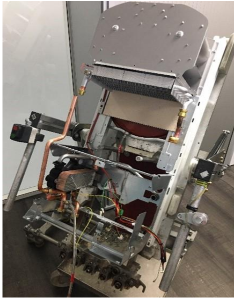
Figure 2-8. Assembled boiler for our case study
