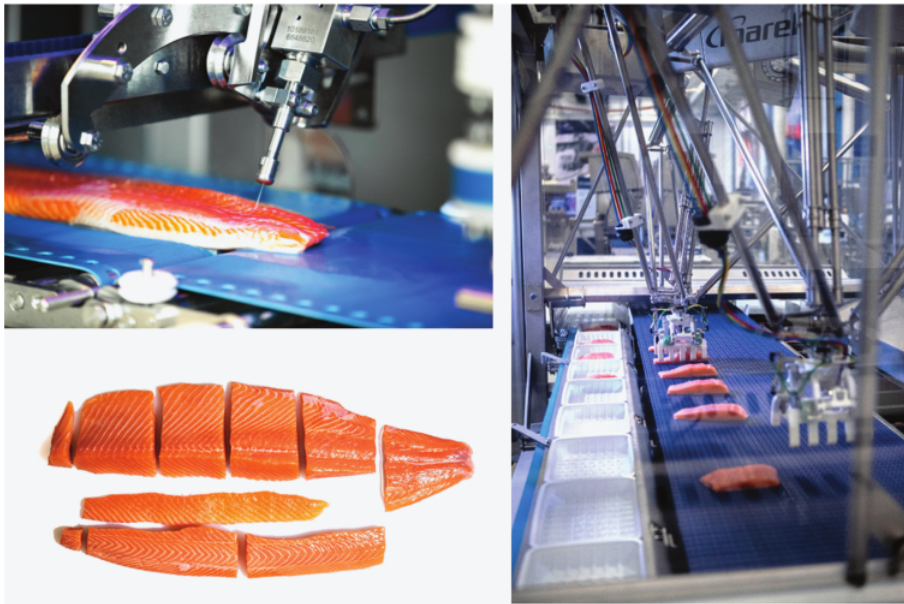
Figure 1.1: An example of automated robotic salmon fillet cutting, from [Einarsdóttir et al., 2022].
