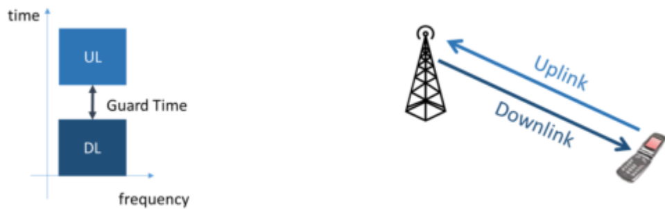
Figure 3.22 – Time Division Duplex principle
