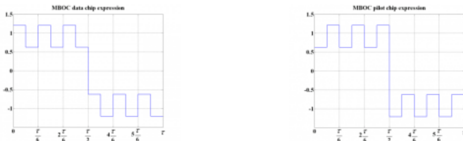
Figure 2.17 – CBOC(6, 1, \frac{1}{11}, +) (left) and CBOC(6, 1, \frac{1}{11}, -) (right) sub carrier time representation – source [19]
