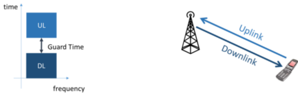
Figure 3.22 – Time Division Duplex principle
