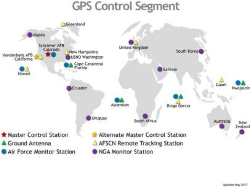
Figure 2.4 – GPS control segment
