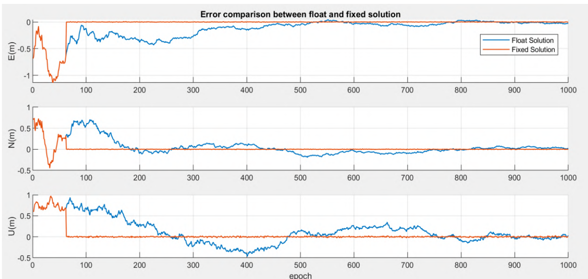
Figure 5-31 Illustration of float vs fixed solution (0 baseline)
