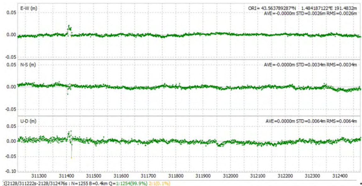
Figure 6-9 Estimation result of RTKLIB for dataset 1
