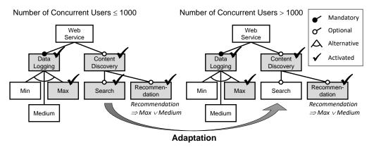
Figure 3.1: Feature model and adaptation of example web service
