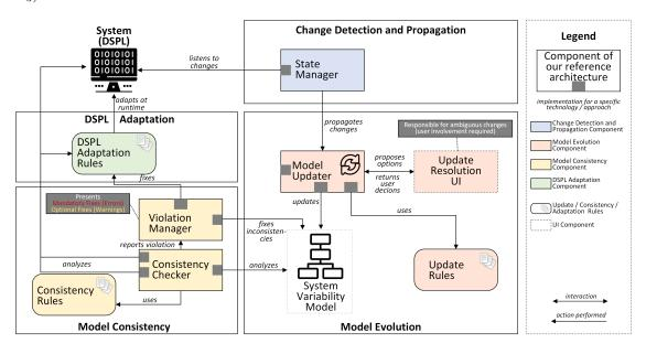
Figure 2.6: Reference architecture for DSPL evolution.
