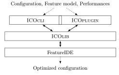
Figure 4.9: The architecture of the ICO tool suite.
