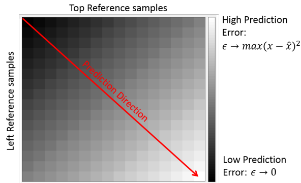
Fig. 3.1 Spatial distribution of the prediction error \epsilon = (x - \hat{x})^2 with x the source sample and \hat{x} the predicted sample, using diagonal-left predictor (mode number 18)
