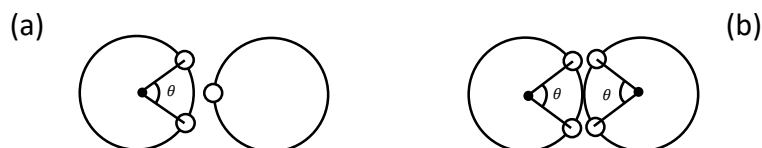
Figure 4.2: (a) Wertheim's SI2W, where a site from one molecule can only be bonded to one site from another molecule. (b) Wertheim's SI2S, where double bonding is not allowed as a consequence of SI1 and SI2W.
