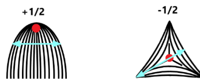
Figure 58. Representation of core (red) and how size is measured (blue arrow) for each defect
