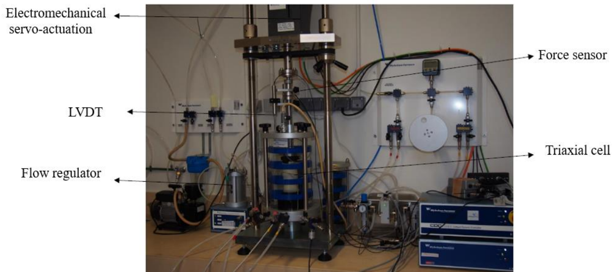
Figure 2.28: Cyclic triaxial test of Antea Group laboratory (Lila, 2021)
