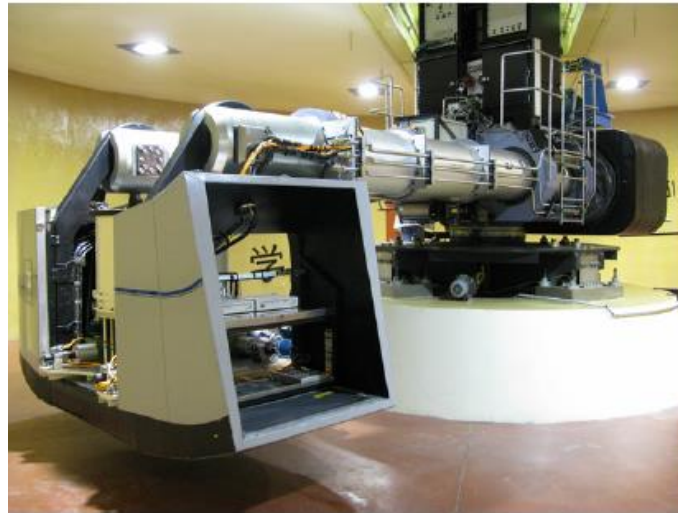
Figure 2.35: Modern centrifuge of the LCPC
