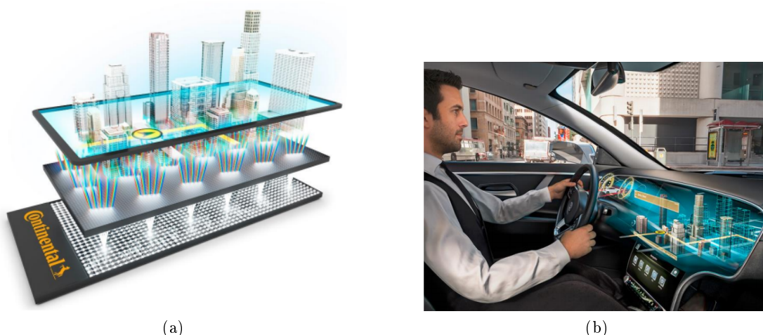
Figure 1.13: (a) Array of microlenses responsible for the angular distribution of light rays and (b) Light Field displays used to render 3D holographic information for drivers.
