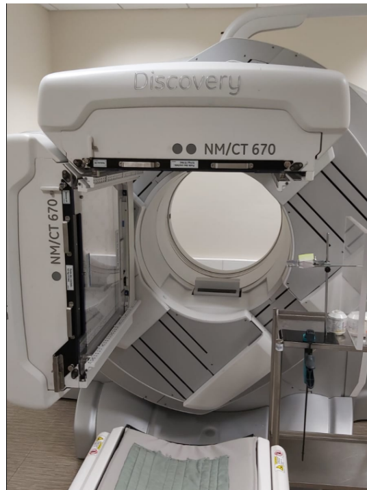
FIGURE 6.1 – Measurement set up to estimate the dead time of the GE Discovery NM/CT 670 gamma camera using the decaying source method. The source is located in a vial attached to a support which is itself attached to a mobile trolley allowing the distance between the source and the detector to be varied.
