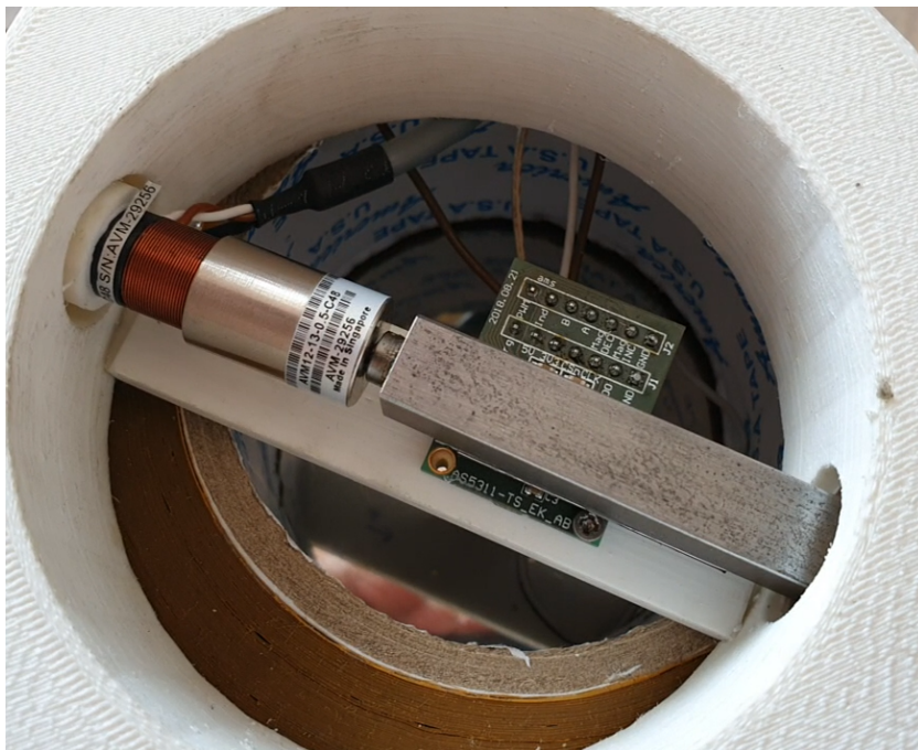
Figure 8.15 Voice Coil on 3d Test Bench
