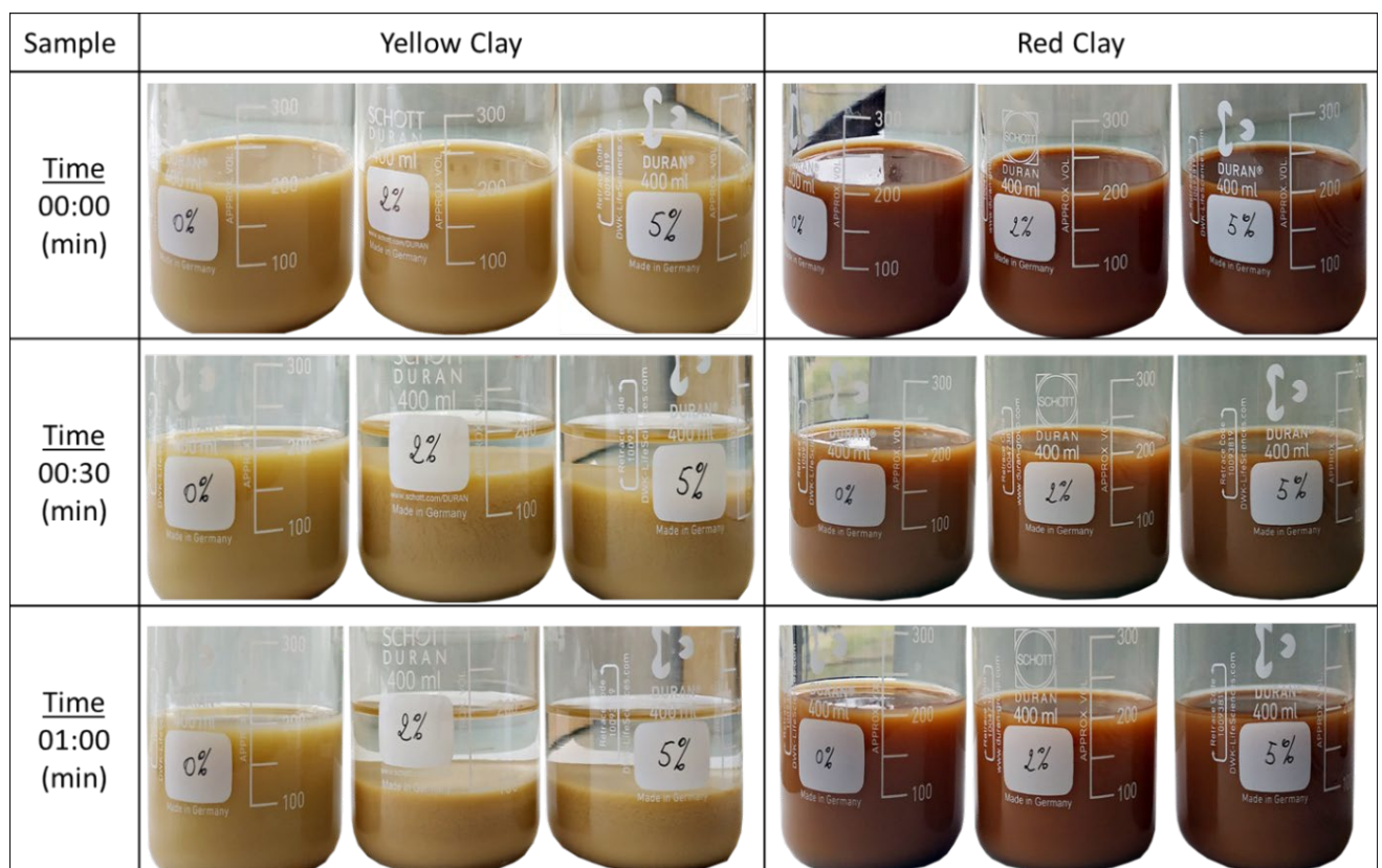
Fig. 39: Laboratory test based on reaction of salt, water and yellow/red clay sediment
