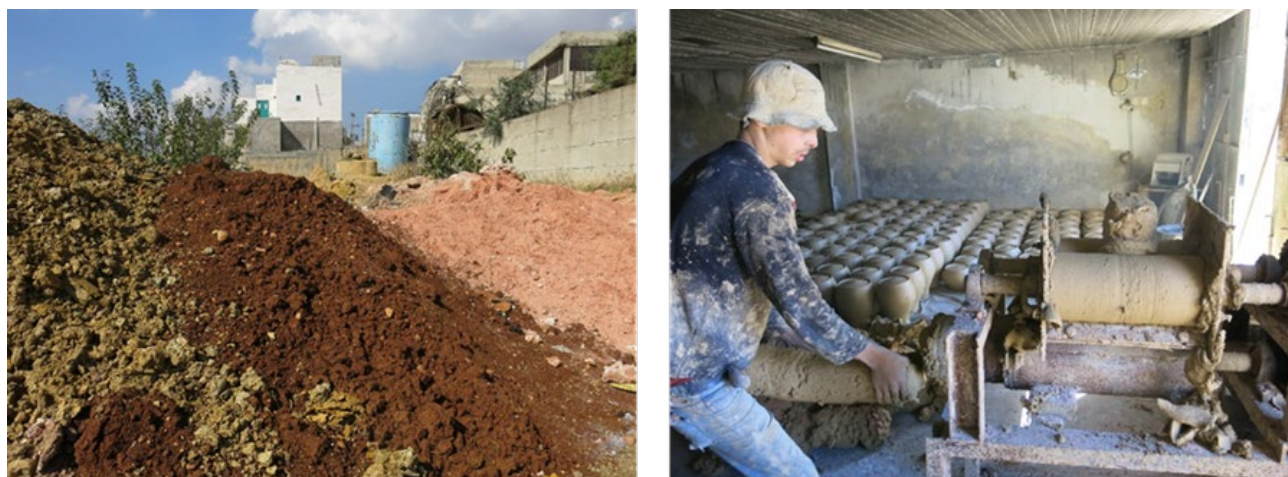
Fig. 35 Raw materials: yellow and red clay sediments and sand (left image); wedging the clay with a pug mill (right image). At this stage the salt is added to the clay material (photographs by V. Roux)
