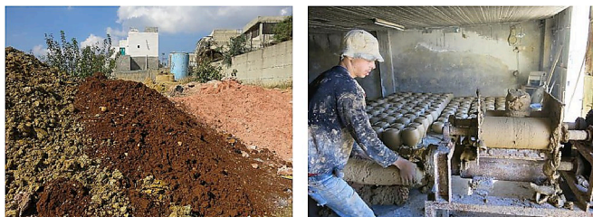
Fig. 1. Raw materials: yellow clay, red clay, and sand (left image). Wedging the clay with a pug mill. It is at this stage that the salt is added to the clay paste (right image). (photographs by V. Roux). (For interpretation of the references to color in this figure legend, the reader is referred to the web version of this article).
