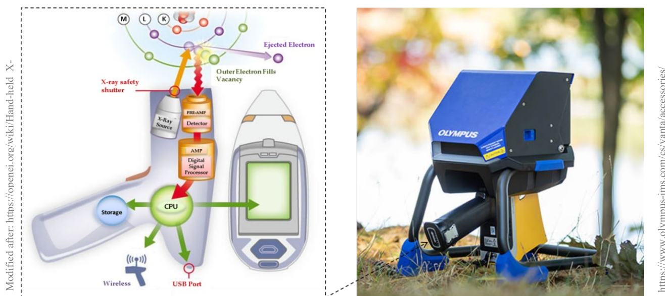
Fig. 16 Schematic diagram of portable XRF analyzer (left image); p-XRF instrument illustration (right image)
