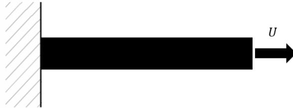
FIGURE 2.8 – Description de l'essai de traction uniaxial
