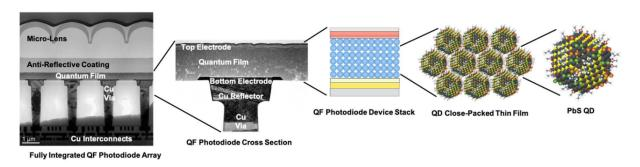
Figure 2: Photodiode array based on NC layers integrated on top of CMOS readout. From left to right are decomposed the different elements. Reproduced from [2].
