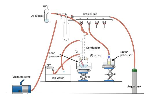
Figure 1.17: Illustration of a synthesis bench.
