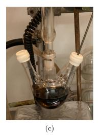
Figure 1.18: Image of the NC PbS synthesis. Resulting solution after the lead precursor complexation at t=0 (a) and t=12 h (b). The final solution that contains the PbS NCs in ODE (c).
