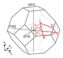
Figure 2.3: First Brillouin Zone of face-centered cubic lattice. Reproduced from [26].
