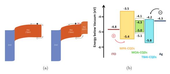
Figure 6.1: (a) Schematic illustration showing the band bending in ZnO/PbS-TBAI (on the left) and ZnO/PbS-TBAI/PbS-EDT (on the right). Reproduced from [47]. (b) The energy level diagram depicts an arrangement of infrared LEDs using NC layers. Within the active NC layer (MOA-CQDs), there are corresponding energy levels for NCs that emit at 1622nm (illustrated by a solid line) and 1220nm (represented by a broken line). Reproduced from [48].
