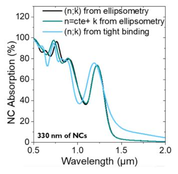
Figure 4.7: Absorption spectra within the NC layer for a diode stack composed of glass/ITO(190 nm)/TiO2(120 nm)/PbS (n-type, with PbS 1200 capped by NH4I), PbS (p-type, with PbS 1200 capped with EDT)/Au (80 nm).
