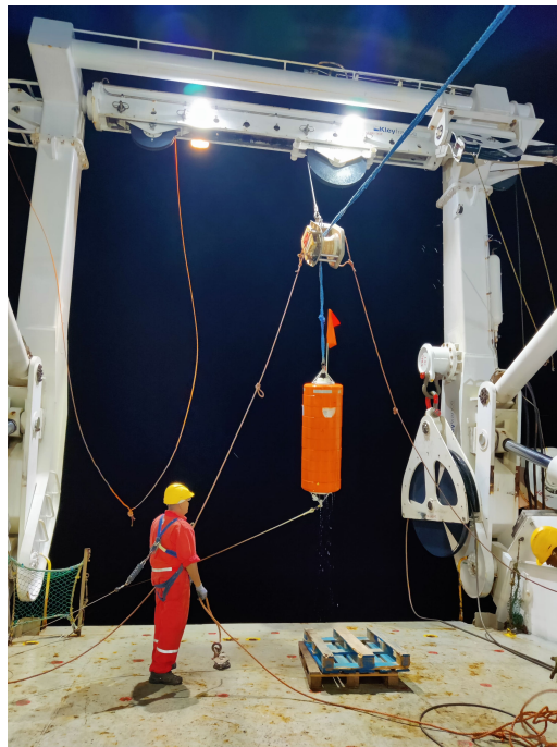
Figure 2.15: Recovery of hydrophone instrument on ship
