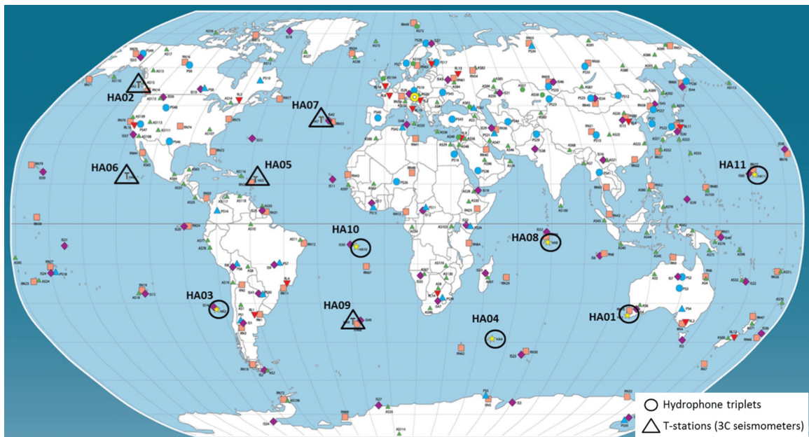
Figure 2.16: Distribution of the IMS-CTBTO worldwide sensor network. The hydro-acoustic stations are comprised of five T-phase stations (black triangles) equipped with three-component seismometers typically deployed on small oceanic islands or close to the coast, and six hydrophone stations (black circles) each composed of triplets of underwater hydrophones, (after Nielsen et al., 2021).
