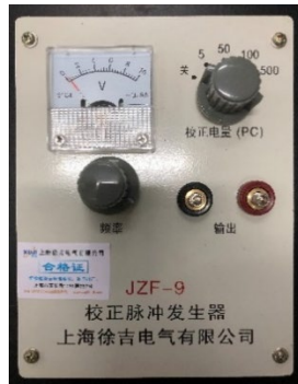
Fig.3.3 JZF-9 type calibration pulse generator
