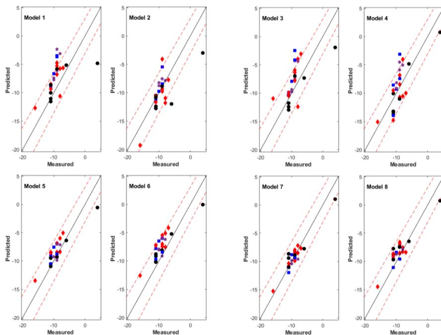
Figure 20. Parity plot for model performance comparison in predicting diesel CFPP in 26 new samples. Red dotted lines: reproducibility limits of the reference method ( $\pm 3 \cdot 0.06 \cdot CFPP$ ). Legend: Black circles  $\rightarrow$  Samples group 1. Red diamonds  $\rightarrow$  Samples group 2. Blue squares  $\rightarrow$  Samples group 3. Purple stars  $\rightarrow$  Samples group 4
