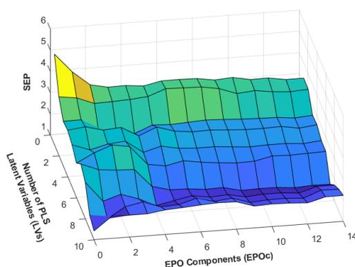
Figure 1. Standard error of prediction on Mx2A as a function of the number of PLS latent variables and EPO components
