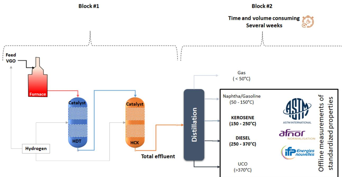
Figure 2. Hydrocracking process global scheme
