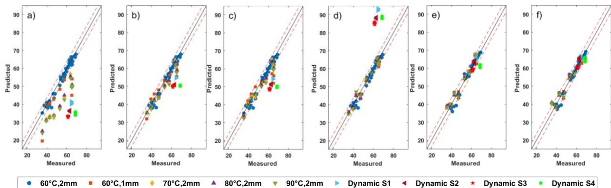
Figure 15. Parity plot for model performance comparison applying external parameters correction. a) reference PLS model b) approach (i) global PDS transfer function, c) approach (i) individual PDS transfer function, d) approach (ii) individual modelling, e) approach (iii) global modelling, f) approach (iv) robust modelling using orthogonalization. Red dotted lines: upper and lower limits of the reproducibility of the reference method
