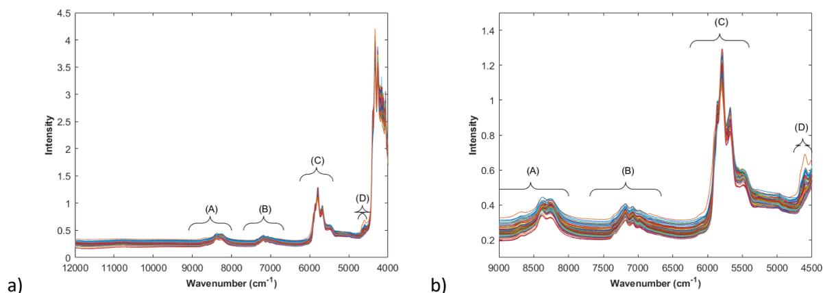
Figure 1. a) NIR spectra full spectral range (12000-4000 cm<sup>-1</sup>), b) NIR spectra spectral range used in modelling (9000-4500 cm<sup>-1</sup>). Identified regions: (A)(9000-8000 cm<sup>-1</sup>), (B)(7600-6600 cm<sup>-1</sup>), (C)(6250-5400 cm<sup>-1</sup>), (D)(5800-4500 cm<sup>-1</sup>)
