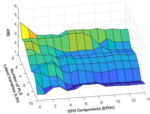
Figure 2. Standard error of prediction on Mx2A as a function of the number of PLS latent variables and EPO components when DOP is applied
