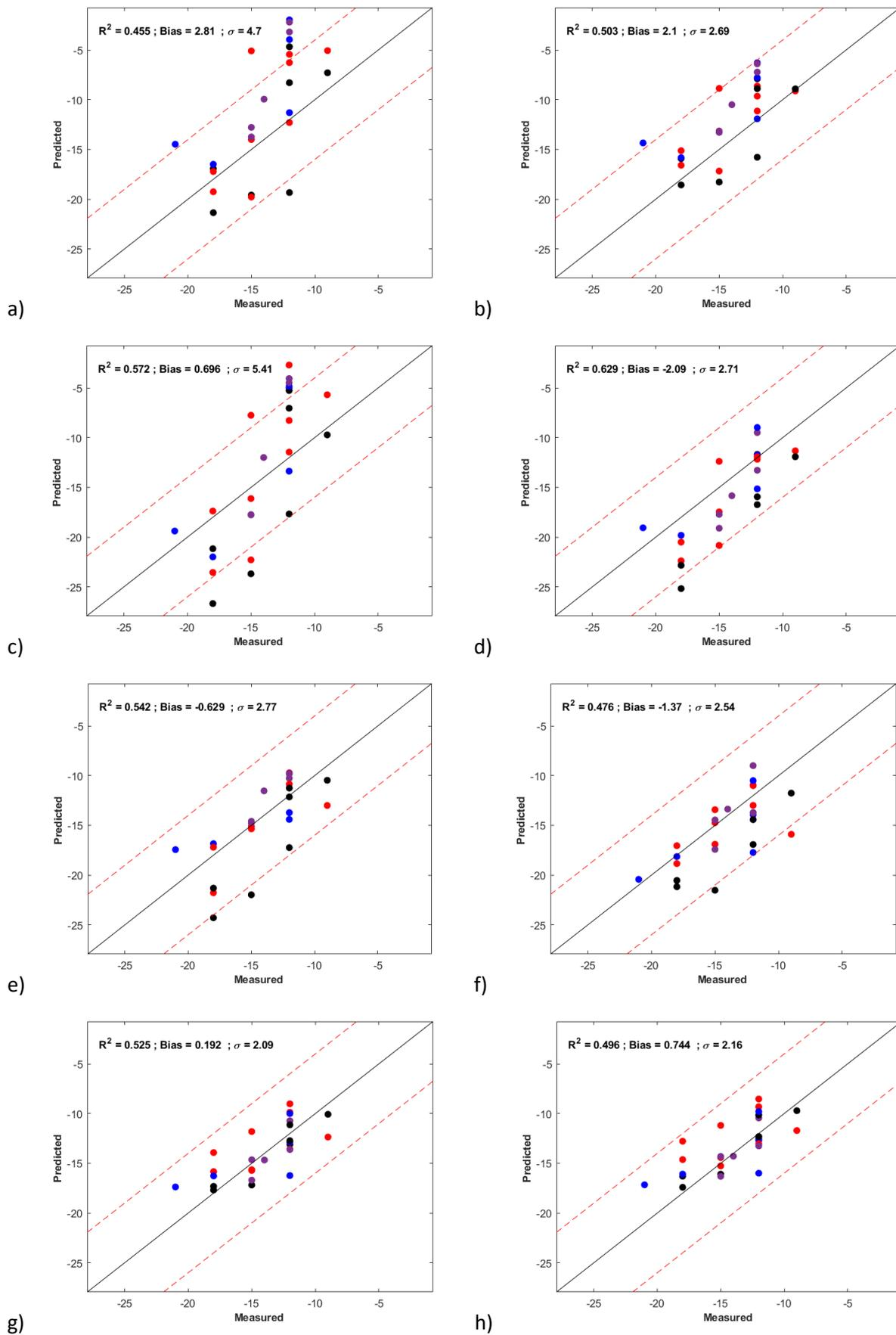
Figure 2 Appendix 7. Parity charts of diesel pour point validation with 26 new samples. a) Model 1, b) Model 2, c) Model 3, d) Model 4, e) Model 5, f) Model 6, g) Model 7, h) Model 8
