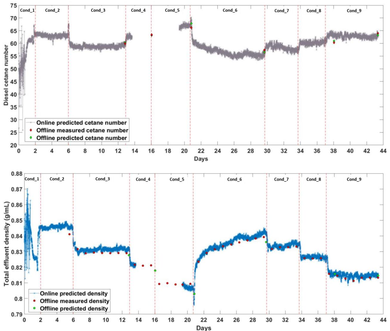
Figure 21. Online HCK process monitoring. Legend → Cond\_1: catalyst sulfiding, Cond\_2: Feedstock A injection, Cond\_3: Feedstock B injection, Cond\_4: Operating temperature increase, Cond\_5: Operating temperature increase, Cond\_6: Feedstock C injection, Cond\_7: Operating temperature increase, Cond\_8: Operating temperature increase, Cond\_9: Operating temperature increase
