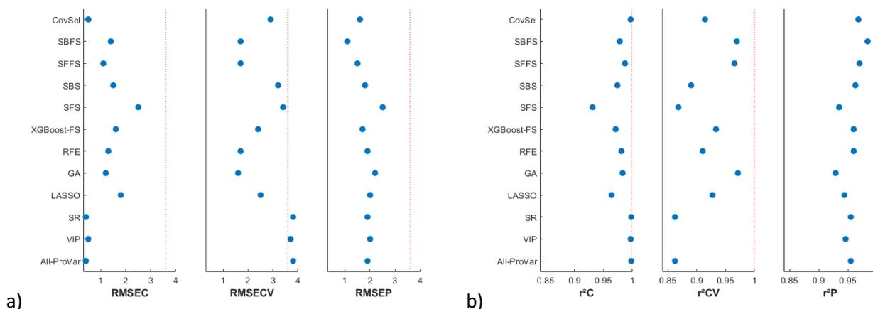
Figure 8. Performance comparison of variable selection methods applied on process variables data block. a) model errors, red dotted line  $\square$  reproducibility of the reference method (3.6). b) model squared correlation coefficients
