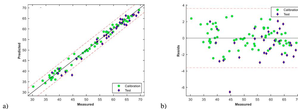
Figure 3. a) Parity plot, b) prediction residuals plot of PLS model for predicting the diesel cetane number
