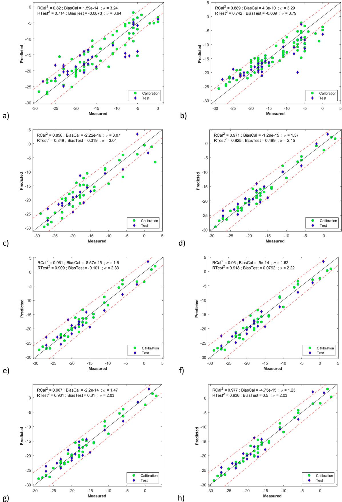
Figure 4 Appendix 6. Diesel cold filter plugging point model parity charts. a) Model 1, b) Model 2, c) Model 3, d) Model 4, e) Model 5, f) Model 6, g) Model 7, h) Model 8
