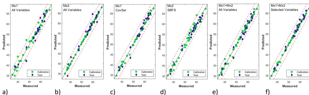
Figure 9. Parity plot for model performance comparison. a) PLS model using all variables from Mx1, b) MLR model using all variables from Mx2, c) MLR model using selected variables from Mx1, d) MLR model using selected variables from Mx2, e) Data fusion model using all variables from Mx1 & Mx2, f) Data fusion model using selected variables from Mx1 & Mx2. Circle shape  $\circ$  calibration samples, diamond shape  $\diamond$  test samples
