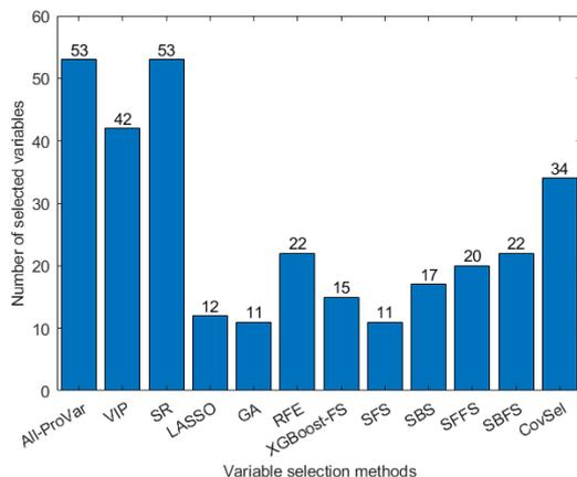
Figure 7. Comparison of the number of selected variables in the process information data block by each method
