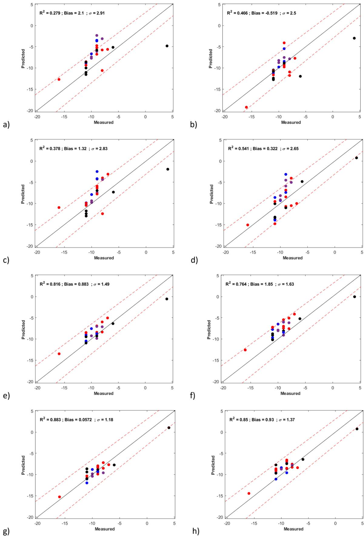
Figure 4 Appendix 7. Parity charts of diesel cold filter plugging point validation with 26 new samples. a) Model 1, b) Model 2, c) Model 3, d) Model 4, e) Model 5, f) Model 6, g) Model 7, h) Model 8
