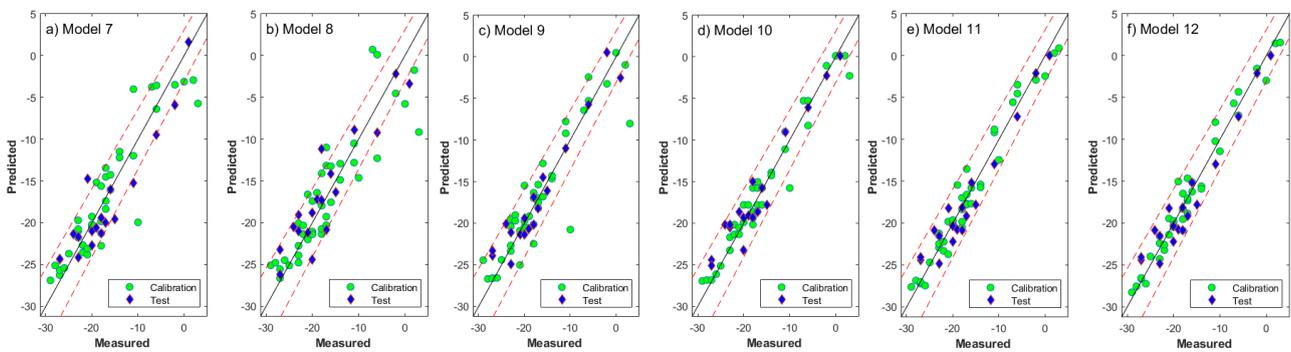
Figure 13. Parity plot for model performance comparison with variable selection. a) MLR model from Mx1, b) MLR model Mx2, c) MLR model from Mx3, d) data fusion model using Mx1+Mx2, e) data fusion model using Mx1+Mx3, f) data fusion model using Mx1+Mx2+Mx3. Red dotted lines: upper and lower limits of the reproducibility of the reference method
