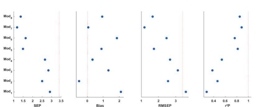
Figure 19. Model performance comparison for predicting diesel CFPP in 26 new samples
