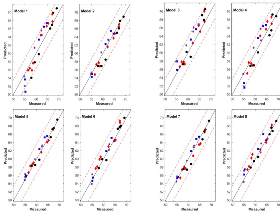
Figure 18. Parity plot for model performance comparison in predicting diesel Cetane Number in 26 new samples. Red dotted lines: reproducibility limits of the reference method ( $\pm 3.6$ ). Legend: Black circles  $\rightarrow$  Samples group 1. Red diamonds  $\rightarrow$  Samples group 2. Blue squares  $\rightarrow$  Samples group 3. Purple stars  $\rightarrow$  Samples group 4
