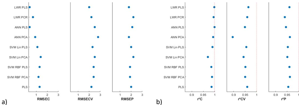
Figure 8. Performance comparison of regression methods employed for diesel cetane number modelling
