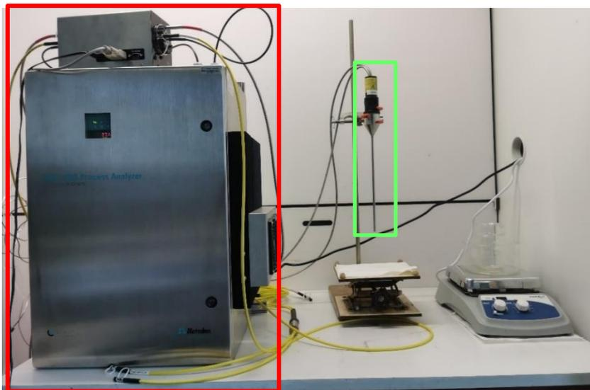
Figure 6. Experimental apparatus employed in the NIR spectra acquisition. Red square → NIR XDS spectrometer, green square → immersion probe
