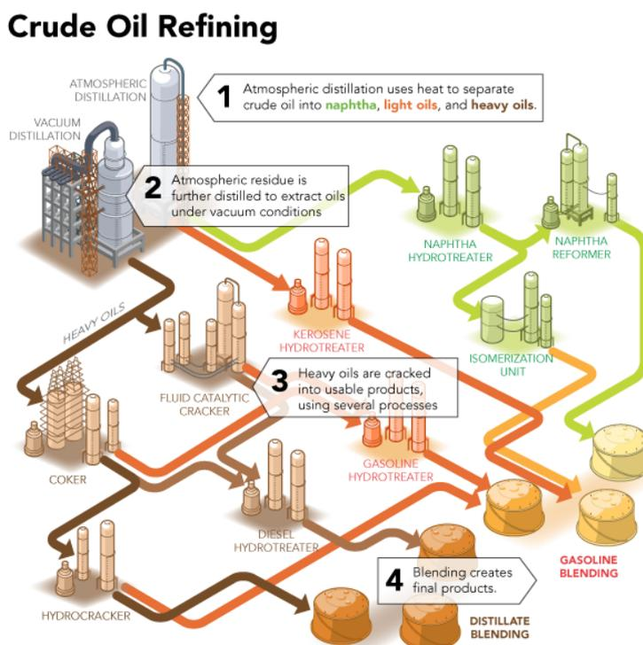
Figure 1. General flow diagram of a refinery
