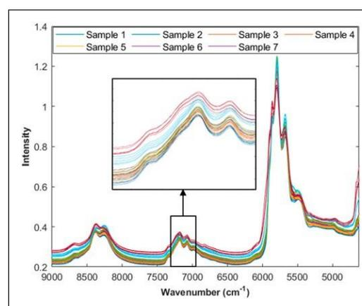
Figure 2. 35 raw spectra used in Case 1 evaluation over the entire spectral range. Legend: Color → samples analyzed. Black square → 35 raw spectra used in Case 1 evaluation magnified over the 7463 cm<sup>-1</sup> - 6993 cm<sup>-1</sup> spectral range.
