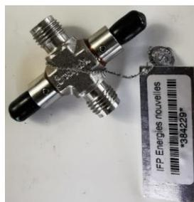
Figure 7. Transmittance Flow cell
