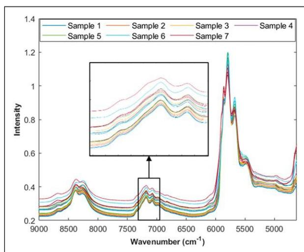
Figure 7. 21 raw spectra used in Case 2 evaluation over the entire spectral range. Legend: Color → samples analyzed. Black square → 21 raw spectra used in Case 2 evaluation magnified over the 7463  $\text{cm}^{-1}$  - 6993  $\text{cm}^{-1}$  spectral range.
