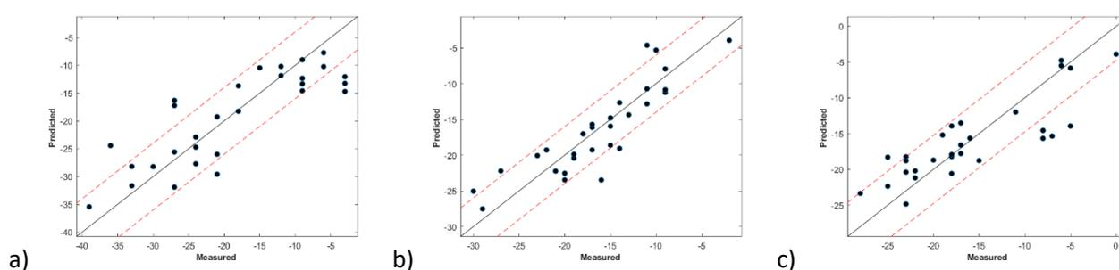
Figure 10. a) Pour Point, b) Cloud Point, and c) Cold Filter Plugging Point parity plot of NIR PLS models
