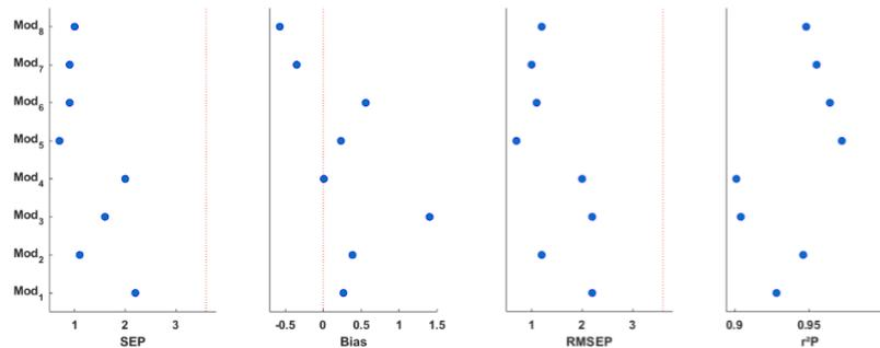
Figure 17. Model performance comparison for predicting diesel Cetane Number in 26 new samples
