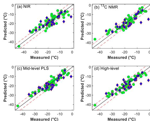
Figure 5. Parity plots of the NIR, <sup>13</sup>C NMR, PLS mid-level, and high-level fusion models for predicting the diesel cloud point (CP). Series legend: circles □ calibration samples, diamond □ test samples. Red dotted lines: upper and lower limits of the reproducibility of the standard method ( $\pm 4^{\circ}\text{C}$ )[5]
