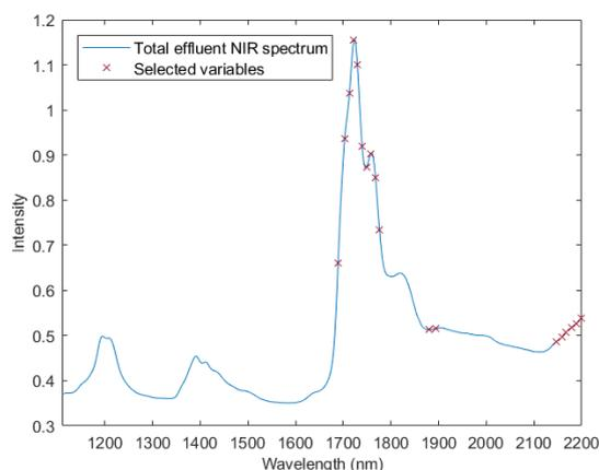
Figure 6. CovSel selected variables identification over an average NIR spectrum acquired on a total effluent sample
