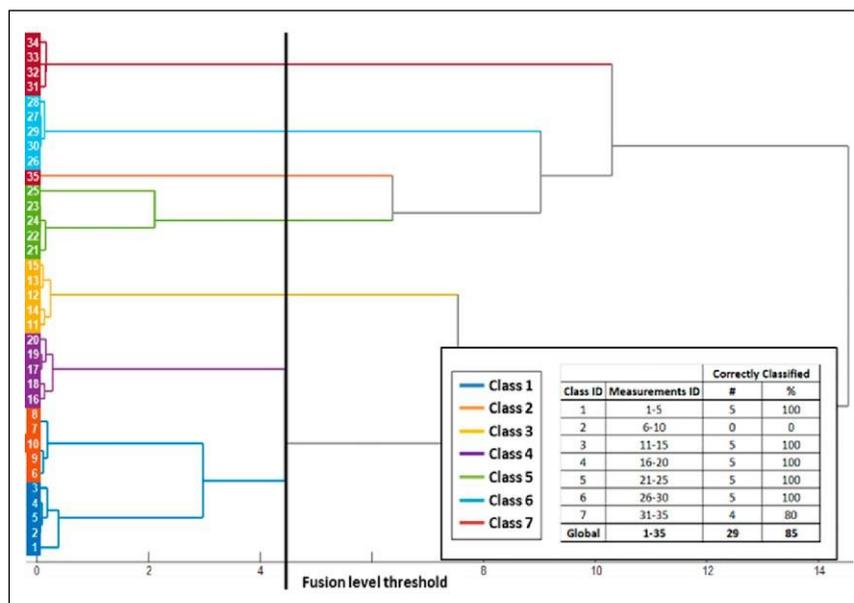
Figure 6. Dendrogram for Case 1 (all measures) with EMSC preprocessing. Legend: Color samples measured (classes). Table: Correct grouping percentage for each class.
