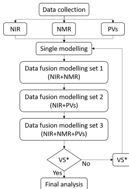
Figure 11. Flow diagram describing the steps involved in improving the NIR model performance. \*VS = Variable Selection applied
