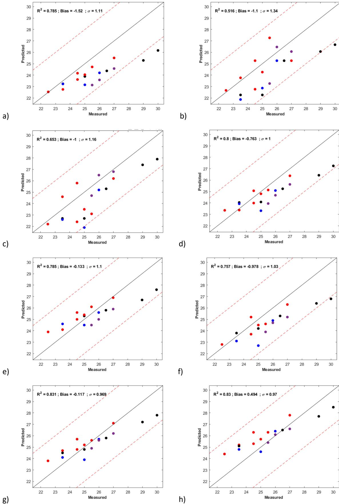
Figure 5 Appendix 7. Parity charts of kerosene smoke point validation with 26 new samples. a) Model 1, b) Model 2, c) Model 3, d) Model 4, e) Model 5, f) Model 6, g) Model 7, h) Model 8
