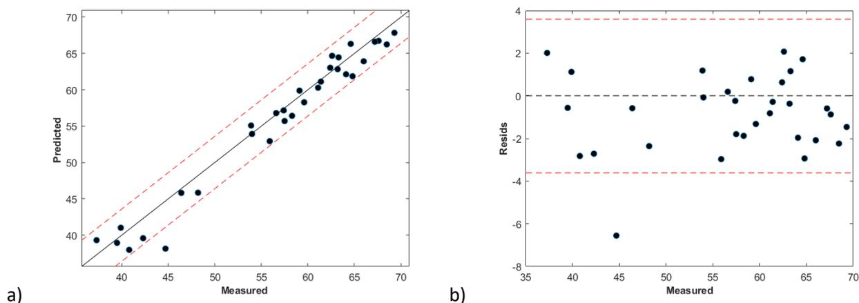
Figure 9. a) Parity plot, b) residuals plot of PLS model for predicting the diesel cetane number from NIR spectra acquired on the hydrocracking total effluent. Red dotted lines: upper and lower limits of the reproducibility of the reference method ( $\pm 3.6$ )
