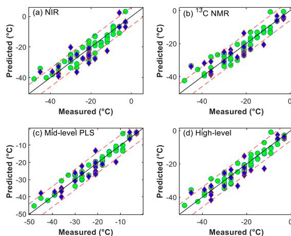
Figure 3. Parity plots of the NIR,  $^{13}\text{C}$  NMR, PLS mid-level, and high-level fusion models for predicting the diesel pour point (PP). Series legend: circles  $\square$  calibration samples, diamond  $\square$  test samples. Red dotted lines: upper and lower limits of the reproducibility of the standard method ( $\pm 6^\circ\text{C}$ ) [4]
