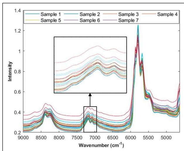
Figure 8. (a) 35 raw spectra used in Case 3 evaluation over the entire spectral range. Legend: Color → samples analyzed. Black square → 35 raw spectra used in Case 3 evaluation magnified over the 7463  $\text{cm}^{-1}$  - 6993  $\text{cm}^{-1}$  spectral range.
