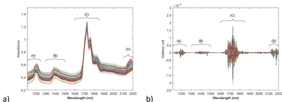
Figure 2. a) NIR spectra in absorbance, b) NIR preprocessed spectra. Spectral range used in modelling (1110-2200 nm). Highlighted regions: (A)(1100-1250 nm), (B)(1300-1500 nm), (C)(1600-1850 nm), (D)(2100-2200 nm)
