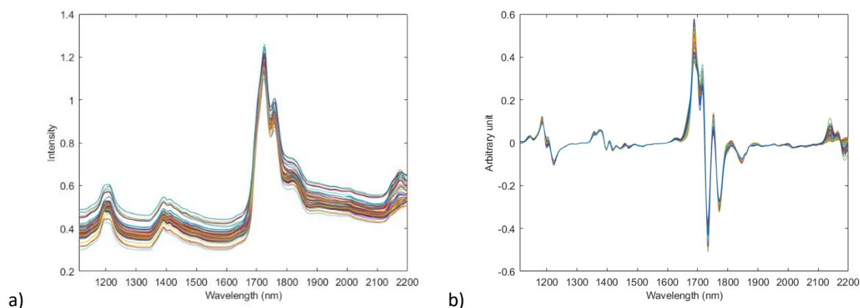
Figure 1. NIR spectra comparison. a) Raw signal, b) preprocessed signal (VSN+SavGol[25,1,1])
