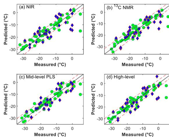
Figure 4. Parity plots of the NIR,  $^{13}\text{C}$  NMR, PLS mid-level, and high-level fusion models for predicting the diesel cold filter plugging point (CFPP). Series legend: circles  $\square$  calibration samples, diamond  $\square$  test samples. Red dotted lines: upper and lower limits of the reproducibility of the standard method ( $\pm(3-0.06*\text{CFPP})^\circ\text{C}$ )[6]
