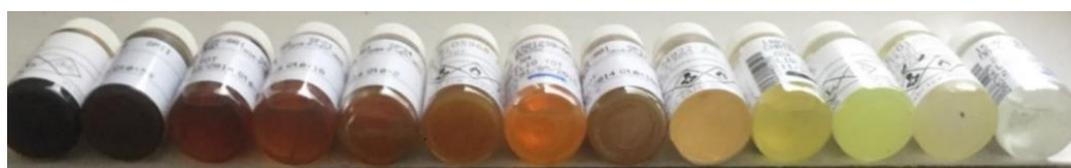
Figure 4. Variability of the color and opacity of total effluent samples obtained from the HCK reactors
