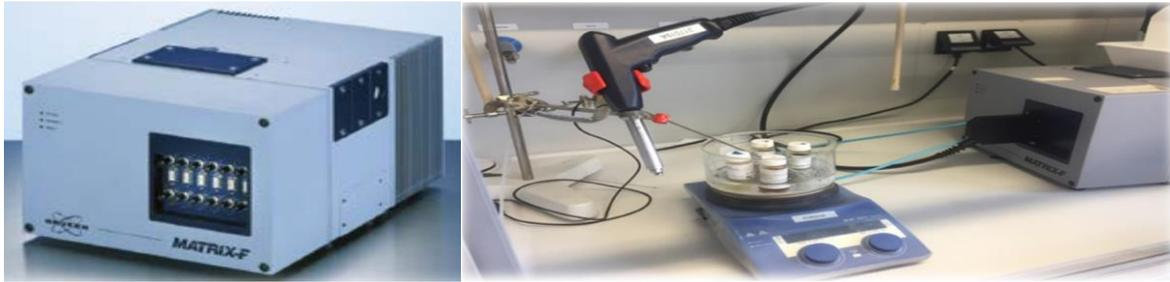
Figure 5. Experimental apparatus employed in the NIR spectra acquisition (Bruker spectrometer)
