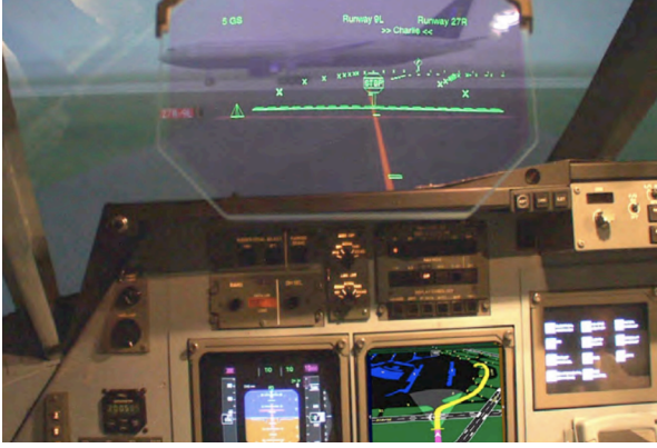
(a) AR system that displays information in front of a pilot in a cockpit [135].
