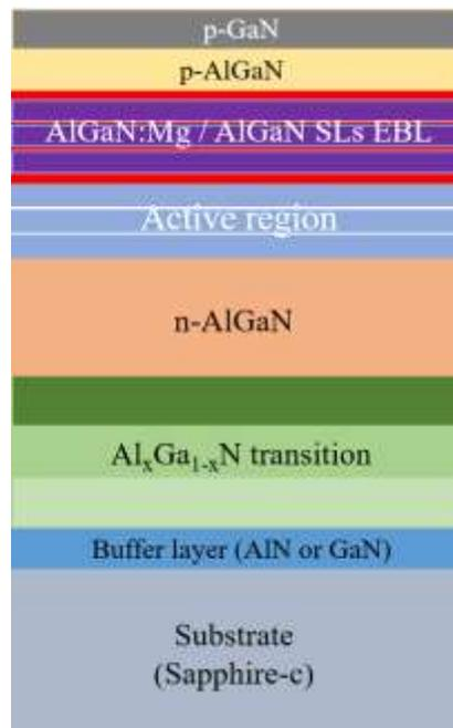
**Figure 27.** Schematic diagram of an LED structure incorporating Mg-doped AlGaN / AlGaN SLs EBL.
