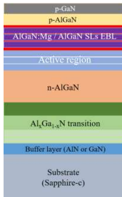
Figure 27. Schematic diagram of an LED structure incorporating Mg-doped AlGaN / AlGaN SLs EBL.
