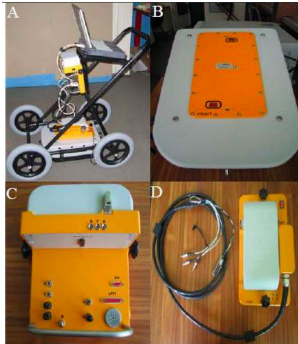
**Figure 4.4:** Radar GPR RAMAC
