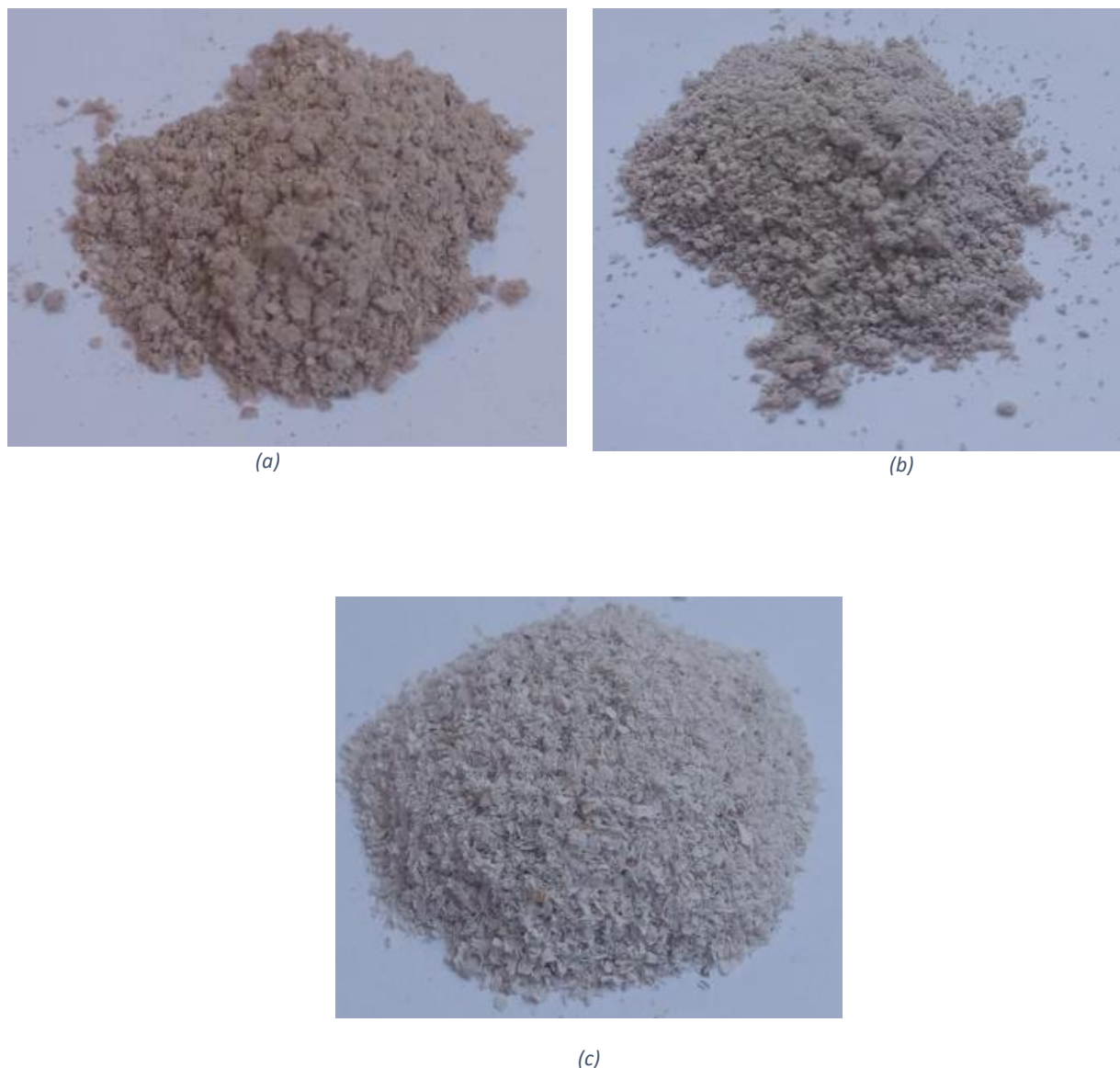
Figure 30. (a) Cassava peels ash (b) Sugar beet pulp ash (c) Ulva lactuca ash.
