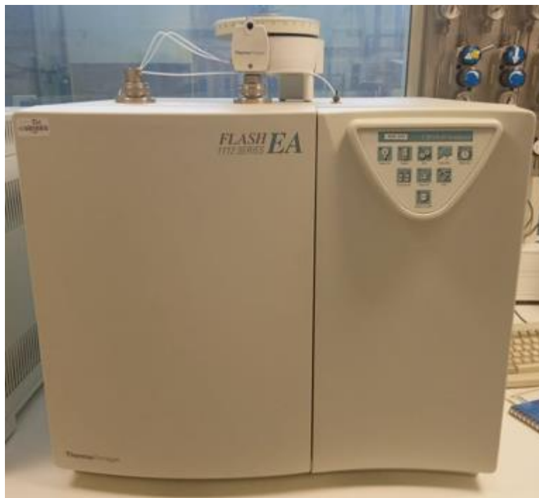
Figure 27. Thermo Finnigan Flash EA 1112 Series CHNS-O Analyser.
