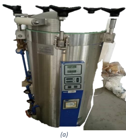
Figure 33. (a) Autoclave verticl 180 liters INOX - Brand: SMI – Used (b) Acid hydrolyzed biomass.
