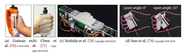
Figure 2.10: Active devices providing feedback within medium warp grasp. (a) Differential skin stretch [76], (b) HaptiVec [77], (c) PoCoPo [78], (d) PaCaPa [79].
