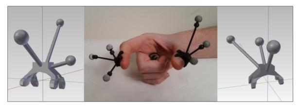
Figure B.4: 3D-printed attachments with constellations of markers. CADs of the thumb and index attachments respectively on the left and right side. A user wearing both in the middle.
