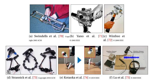
Figure 2.9: Active devices providing feedback non-limited to the hand. (a) TorqueBar [70], (b) Gyro Effect [71], (c) iTorqU 2.0 [72], (d) Haptic Link [73], (d) Physical Contact Feeling of Virtual Objects [74], (e) Rendering Sounds [75].
