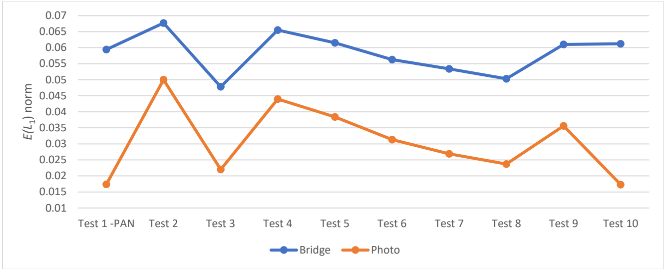
Figure 2: E(L_1) norm variation using ten different regularization parameters combinations for the "Bridge" and "Photo" images, with PSF support size 13 \times 13
