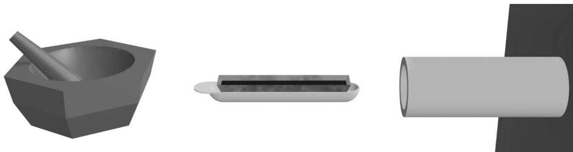
**Figure II.1.** Scheme of the tools used for the ceramic method. From left to right: agate stone mortar, alumina basket with platinum foil and tubular furnace.
