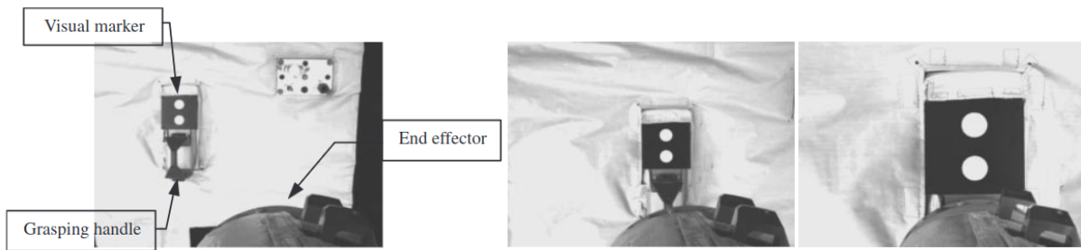
Figure 2.9 – Camera view during visual servoing from [Inaba et al., 2003]. The end-effector is perfectly converging to the grasping handle thanks to the visual positioning task.
