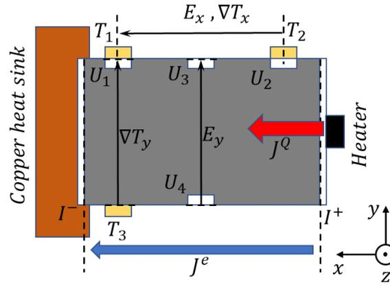
Fig. 1.2 Sketch of the setup that allows to measure the three tensors  $\bar{\sigma}$ ,  $\bar{\kappa}$ , and  $\bar{\alpha}$  at the same time.  $T_1$ ,  $T_2$  and  $T_3$  are three Cernox CX-1030 thermometers. The heater is a  $1\text{ K}\Omega$  chip resistor. All connections on the sample were made using silver paste. Six tin pads (white rectangles) are soldered on the sample for ohmic contacts.
