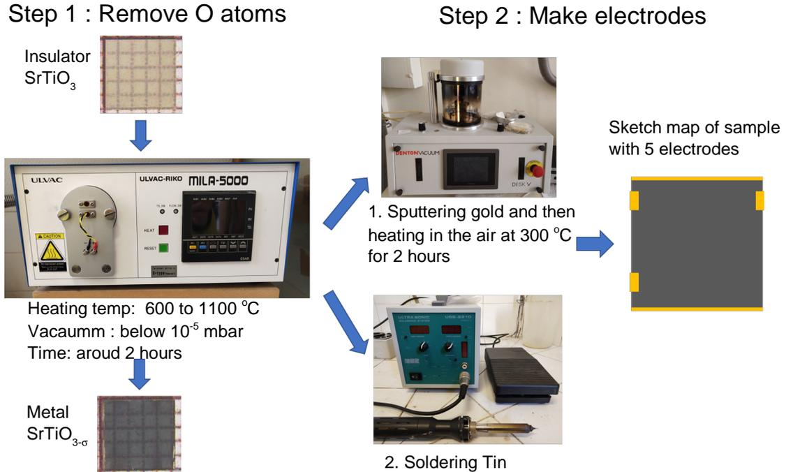
Fig. 3.3 The process of preparation metallic  $\text{SrTiO}_{3-\delta}$  samples.
