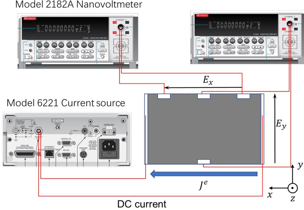
Fig. 1.4 Measurement of the longitudinal and transverse electric field  $E_x$  and  $E_y$  along the sample. Model 6221 provides a DC current along the  $x$  axis.  $E_x$  and  $E_y$  are detected by two Model 2182A nanovoltmeters in the same time
