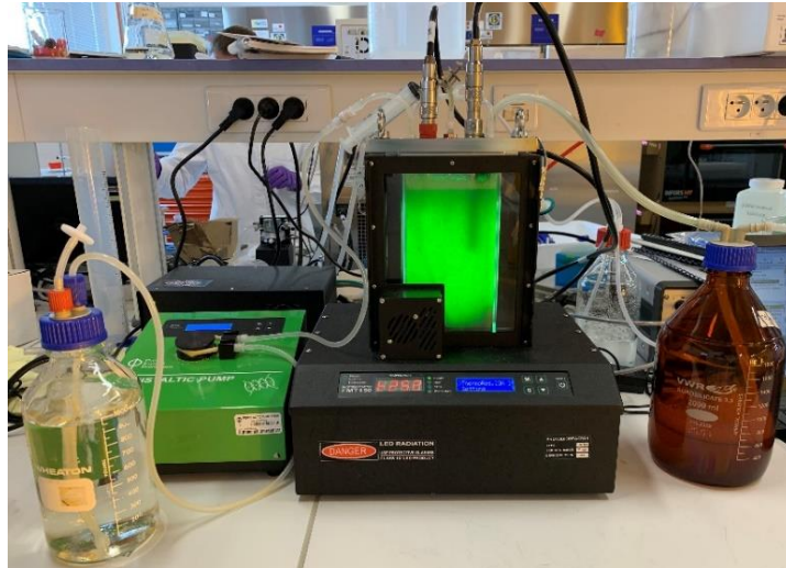
Figure 2. 11. Photobioreactor used for turbidostat cultivation in Paper III.
