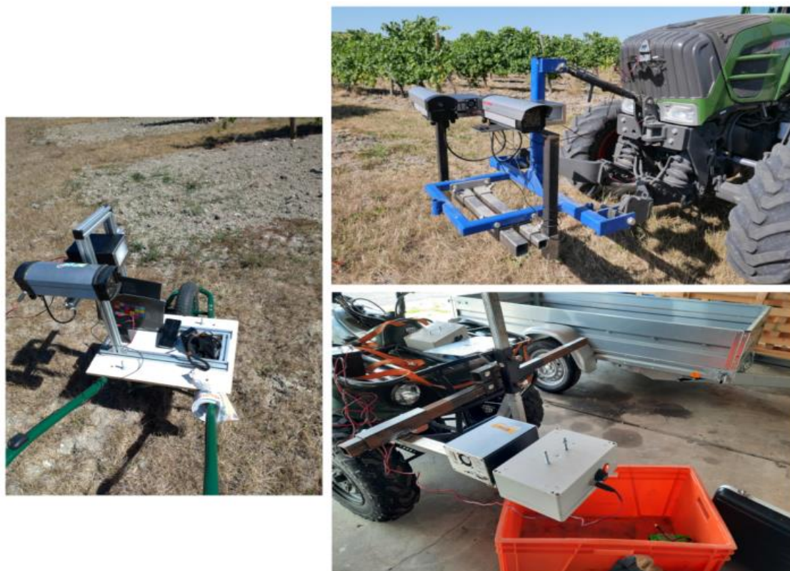
Figure 6. Image acquisition device for the acquisition of FD images attached to a wheelbarrow for targeted acquisitions, a tractor and a quad during automated image acquisitions.
