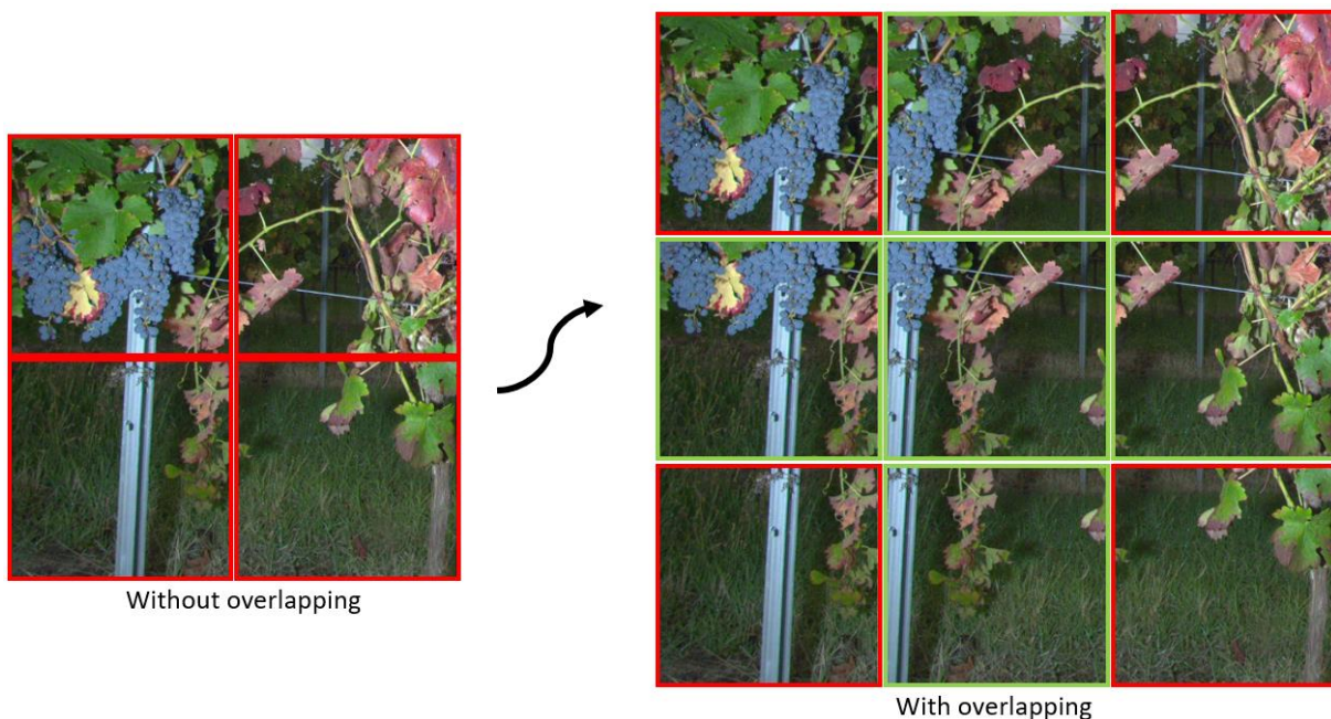
Figure 25. Thumbnail creation with/without overlapping. The thumbnails bordered in green are those created with overlapping.
