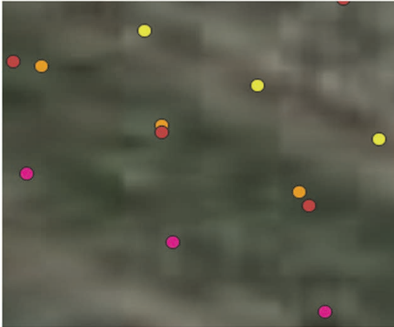
Figure 14. Illustration of the PPK correction and the repositioning of the coordinates at the location of the grapevine photographed. The yellow and pink dots are the uncorrected coordinates of images of the same grapevine row acquired on either side of the row. The orange and red points correspond respectively to the corrected coordinates of the yellow and pink points.
