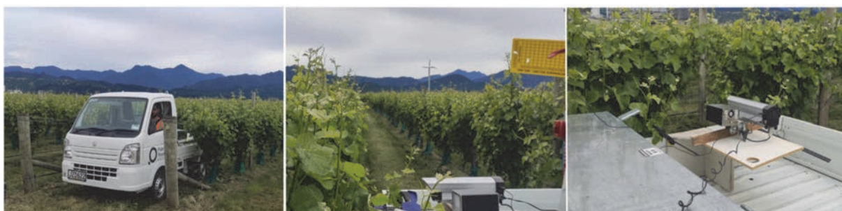
Figure 7. Presentation of the acquisition device attached to the back of a van, remotely controlled via WiFi.
